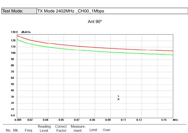
MHz dBuV dΒ dBuV/m dBuV/m dΒ Detector Comment 1 \* 0.1011 12.31 15.97 28.28 107.51 -79.23 QP
