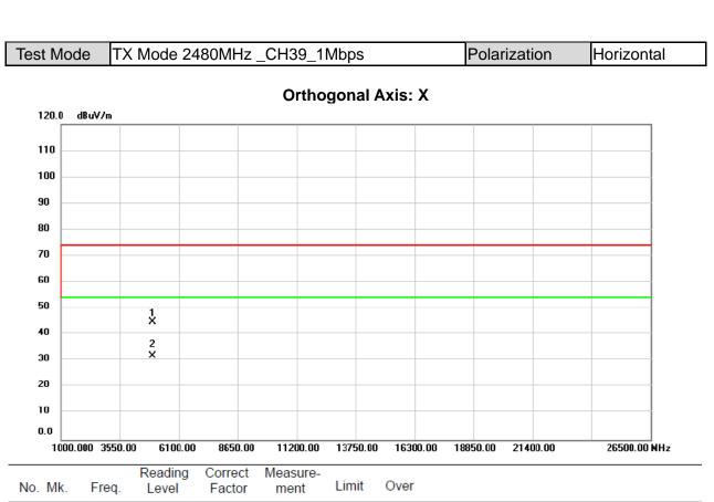
MHz dBuV dΒ dBuV/m dBuV/m dB Detector Comment 1 4960.000 56.29 -11.43 44.86 74.00 -29.14 peak 4960.000 43.49 -11.43 32.06 54.00 -21.94 AVG 2
