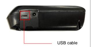
Open the interface cover and connect the printer to the computer with USB cable.
