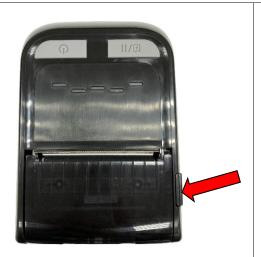
Insert battery to the left side of battery slot on the rear of the printer.
