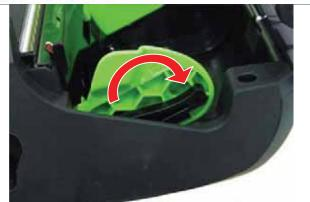
2. Push down each side of media holder lock switch to fix the media holder.
