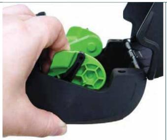
Open the printer media cover by pressing the media cover release button. Pull the media holders apart to fit the media width.
