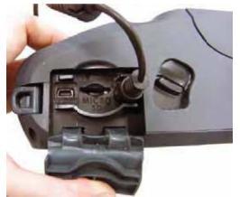
2. Open the interface cover and plug the power cord to the power jack.
