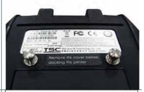
2. Pull up the belt strap to lock it on the screws.
