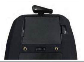
1. The battery is installed into the printer.
