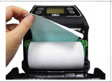
3. Place the roll between the media holders and close them onto the core. Place the paper, printing side face up, and pull out enough paper over the print head.
