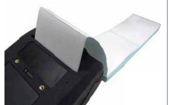
3. Feed the media through the rear external label entrance chute. Place the paper, printing side face up.
