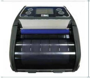
Press each side of media cover to close the media cover and make sure the media cover closed correctly.
