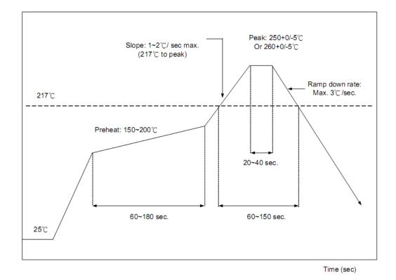
Figure 12: Typical Lead-free Re-flow Solder Profile
