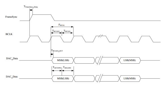
Figure 11: PCM Interface (Short FrameSync)
