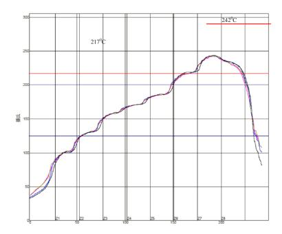
Figure 13 : Typical Lead-free Re-flow
