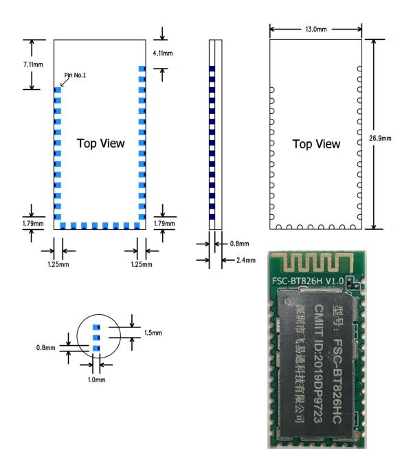
Figure 2: Package Dimensions (TOP VIEW)
