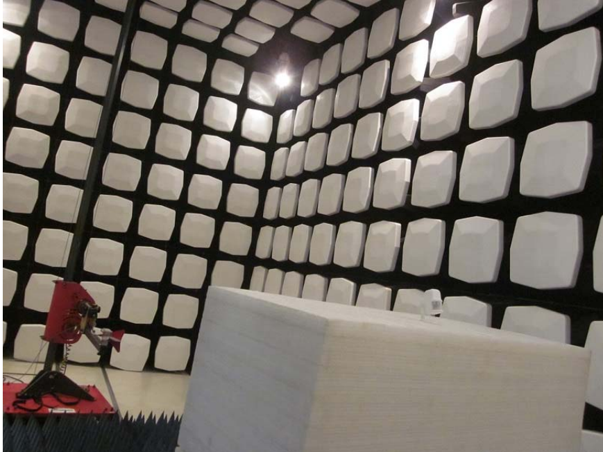
Measurement of Radiated Emission Test Set Up
