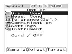
Use the △ or ▽ button of the cross key to move the cursor to "Communication" and then press the [SAVE/SEL] button.
