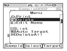
2 Use the < button of the cross key to move the cursor to "OK" and press the [SAVE/SEL] button. Data will be deleted.
