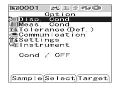
2 Use the △ or ▽ button of the cross key to move the cursor to "Communication" and then press the [SAVE/SEL] button.
