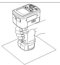
3 Make sure that **≰** (Ready to measure) is displayed or Ready lamp is green, and then press the measuring button.
