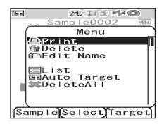
2 Use the △ or ▽ button of the cross key to move the cursor to an item to select or execute, and then press the [SAVE/SEL] button.
