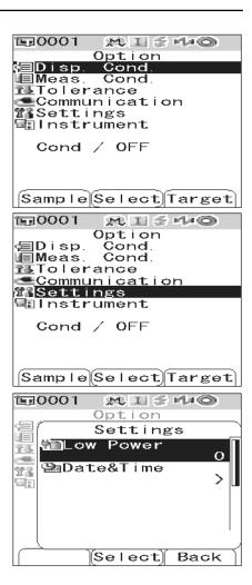
4 Use the △ or ▽ button of the cross key to change the time before the power save mode is activated by specifying the number of minutes.
