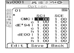
To set each parameter 1, c and h for CMC, ΔE\*94 and ΔE00, place the cursor on the item and press the
