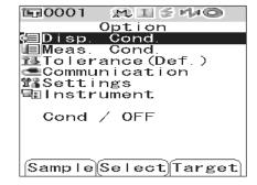
2 Use the △ or ▽ button of the cross key to move the cursor to "Instrument" and then press the [SAVE/SEL] button.
