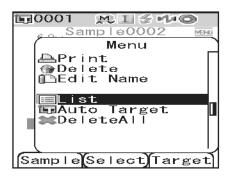
To return to the <Sample> screen, press the [MENU] button while the <Menu> screen is displayed.
