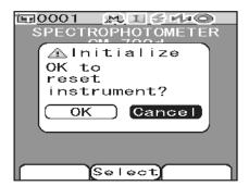
2 Use the ⊲ or ⊳ button of the cross key to move the cursor to "OK" and then press the [SAVE/SEL] button.
