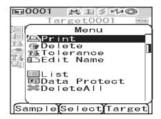
Use the △ or ▽ button of the cross key to move the cursor to "Tolerance" and then press the [SAVE/SEL] button.
