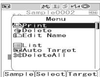
Press the [SAVE/SEL] button. The <Print> screen is displayed and the data is printed from the connected printer.
