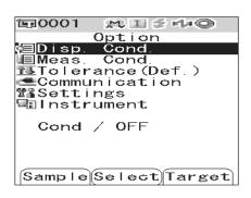
2 Use the ∇ button of the cross key to move the cursor to "Settings" and then press the [SAVE/SEL] button.
