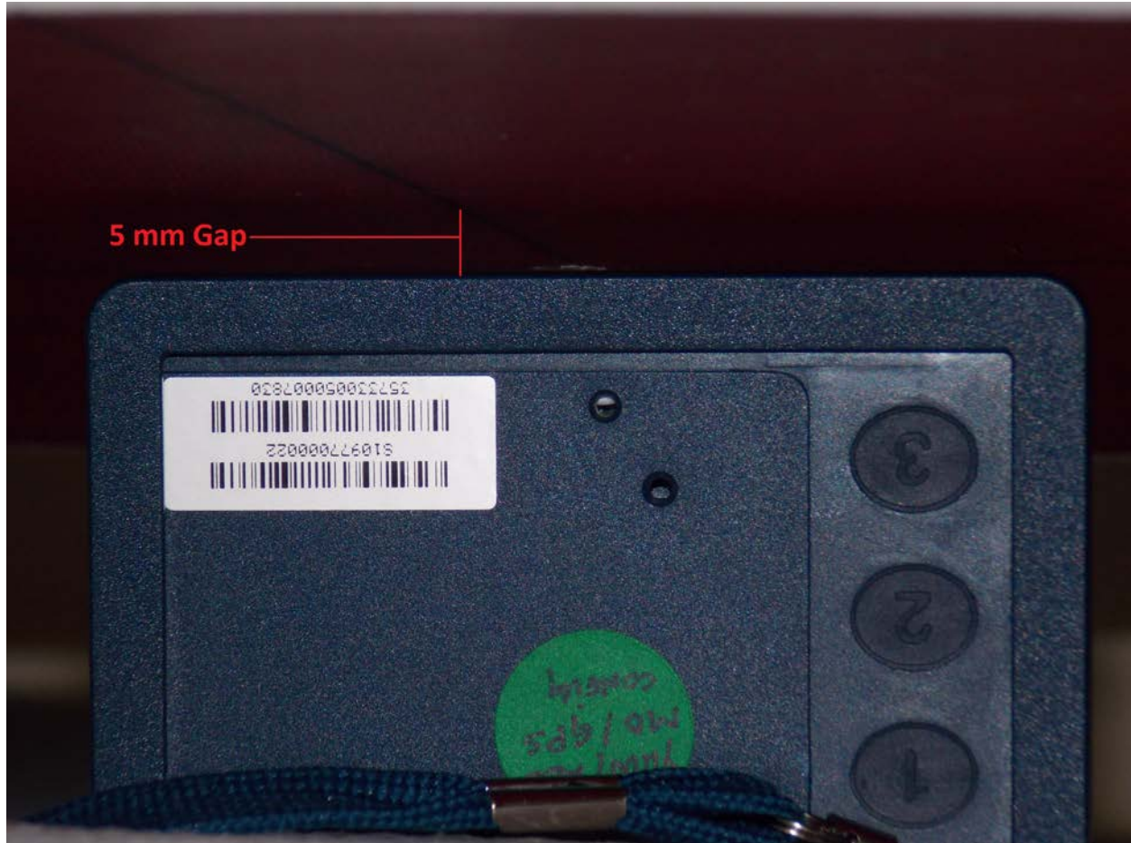
Test Position Side F with Lanyard 5 mm Gap
