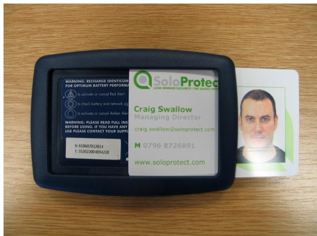
Identicom unit with ID card half inserted
