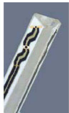
Figure 3.3 Probe Thick-Film Technique
