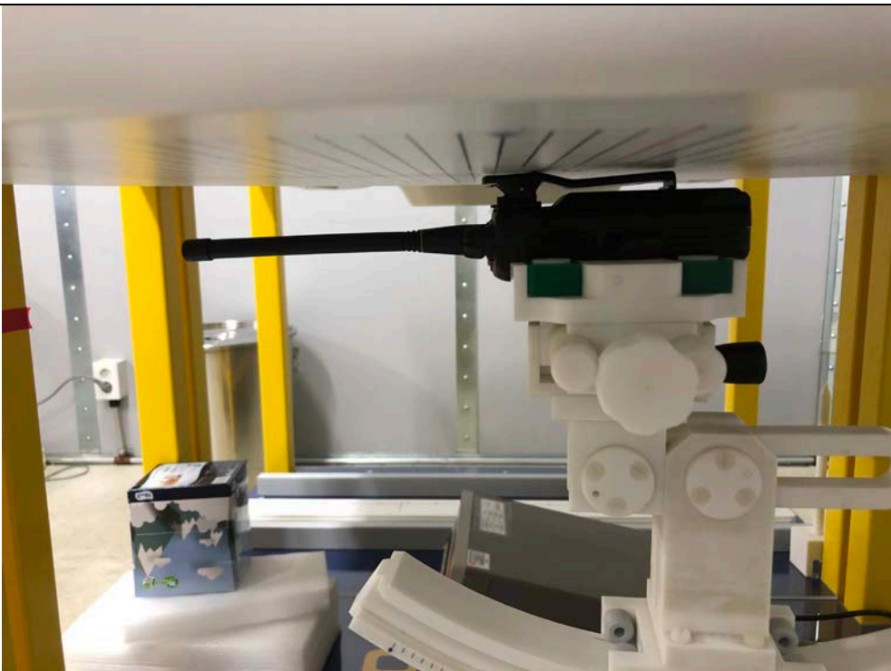
Rear of Device 0 mm from Phantom Side view
