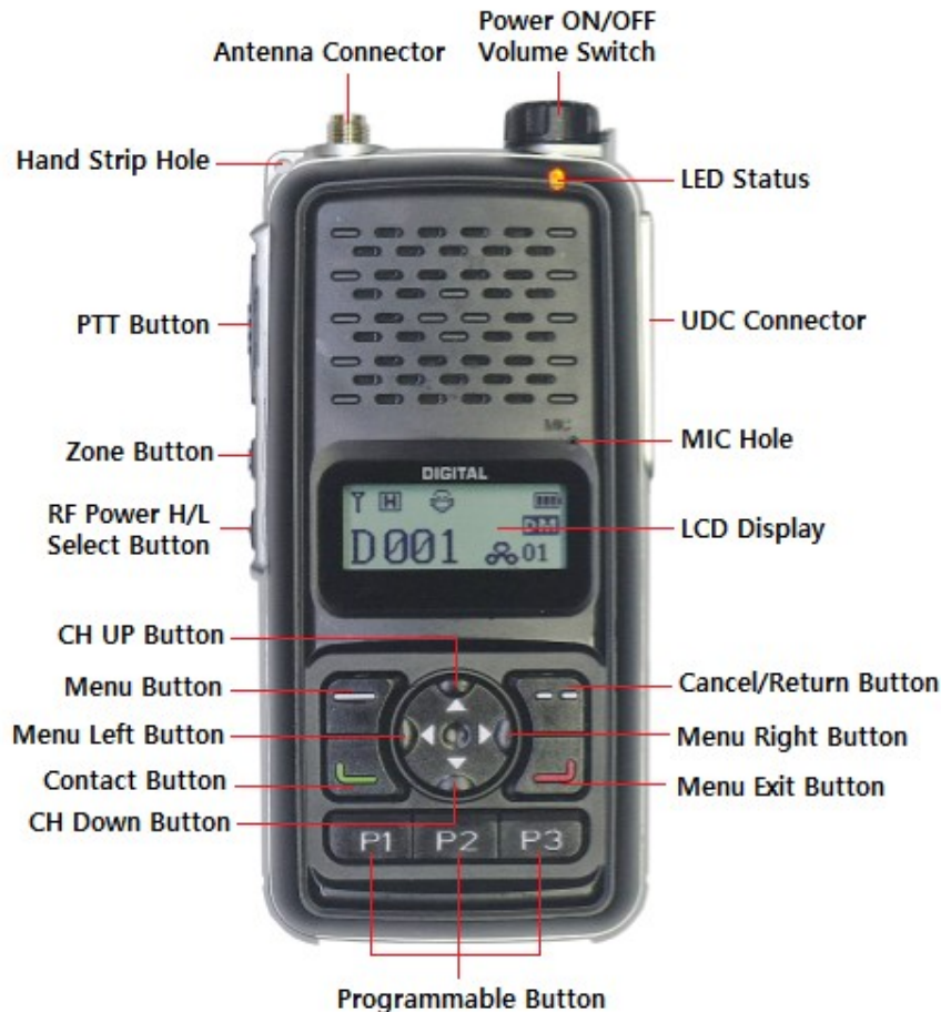
Figure 5-1) DX Series Button Description
