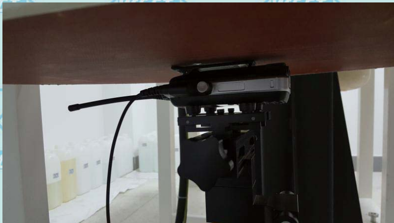
Body-worn, the front of the EUT towards ground with A1, BC1 and AC1 (The distance was 0mm)
