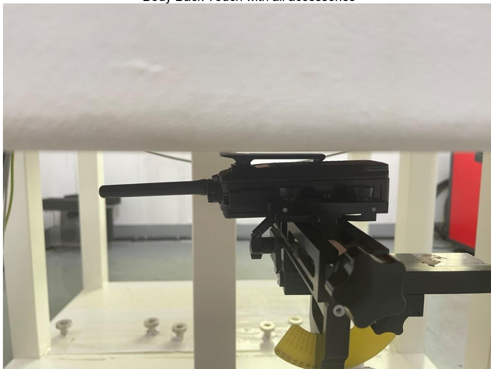
The thickness of EUT is 3.6 cm
