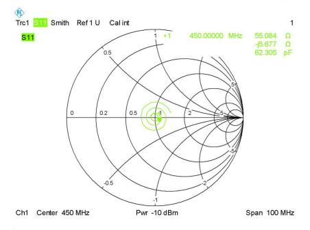
Calibrated return loss: -22.6dB; Measurement return loss: -22.3 dB(within 20%)
