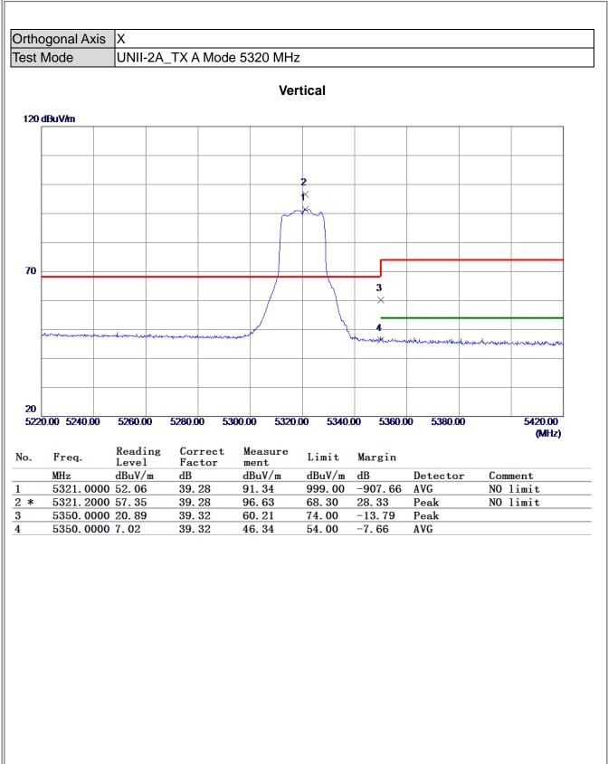
(1) Measurement Value = Reading Level + Correct Factor.
