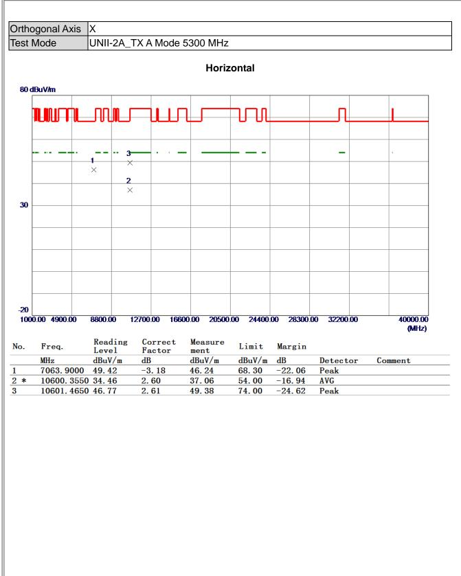
(1) Measurement Value = Reading Level + Correct Factor.
