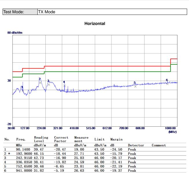
REMARKS: (1) Measurement Value = Reading Level + Correct Factor. (2) Margin Level = Measurement Value - Limit Value.
