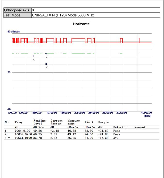
(1) Measurement Value = Reading Level + Correct Factor.
