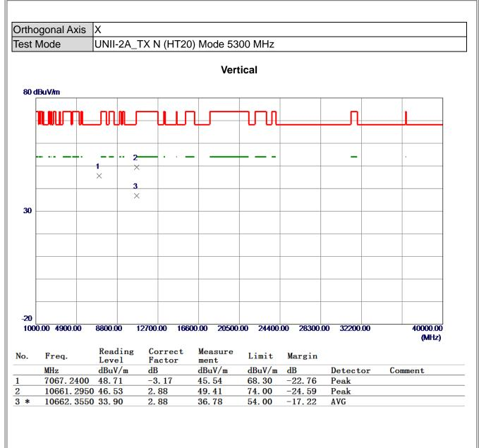
(1) Measurement Value = Reading Level + Correct Factor.
