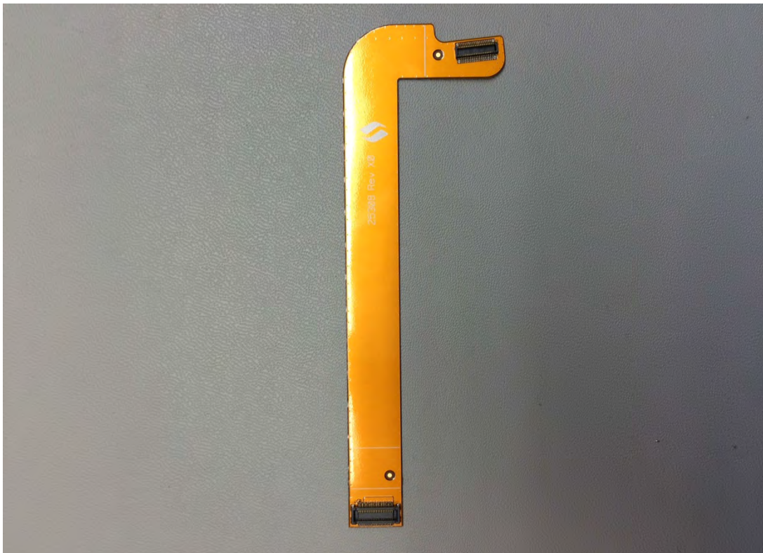
MS2 battery connector flex (back)
