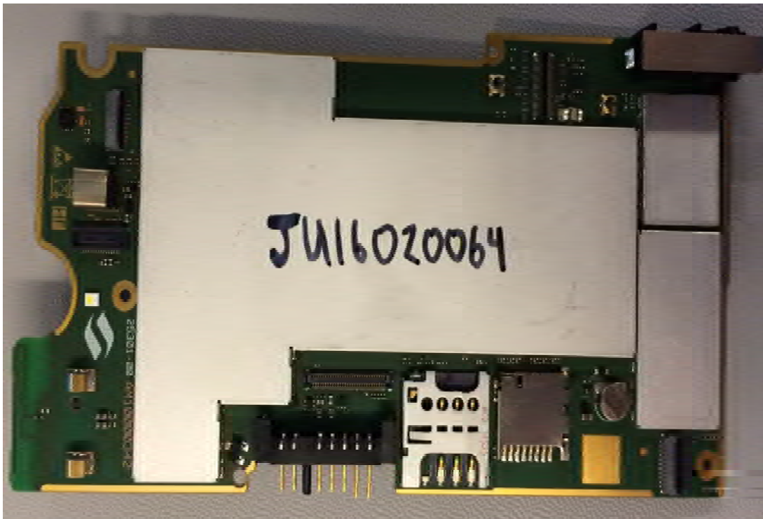
MS2 main PCBA (front) with shields
