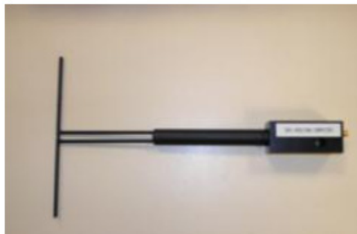
Figure 1 – Satimo COMOSAR Validation Dipole
