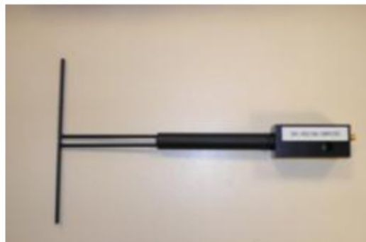
Figure 1 – Satimo COMOSAR Validation Dipole
