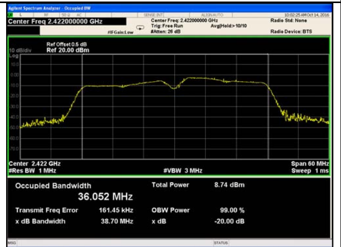
802.11n40 20dB Bandwidth - Low CH 2422
