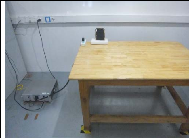
Conducted Emissions Test Setup Front View
