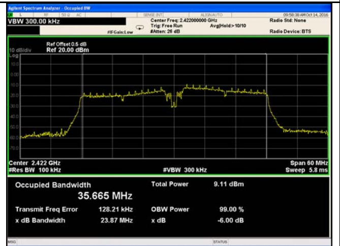
802.11n40 6dB Bandwidth - Low CH 2422
