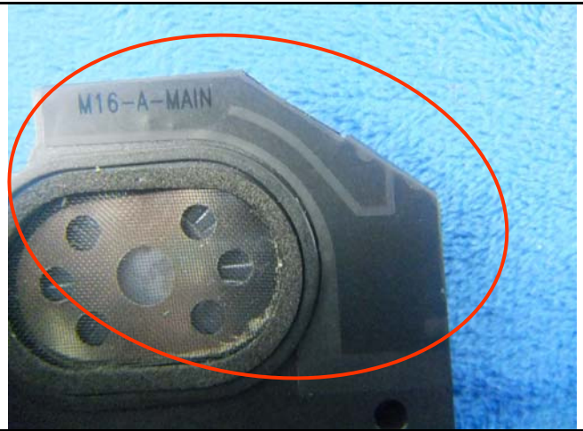
GSM/PCS/UMTS-FDD Antenna View
