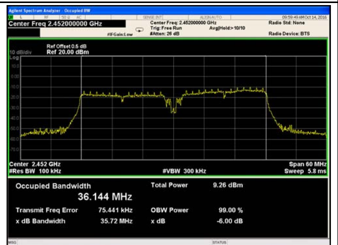
802.11n40 6dB Bandwidth - High CH 2452
