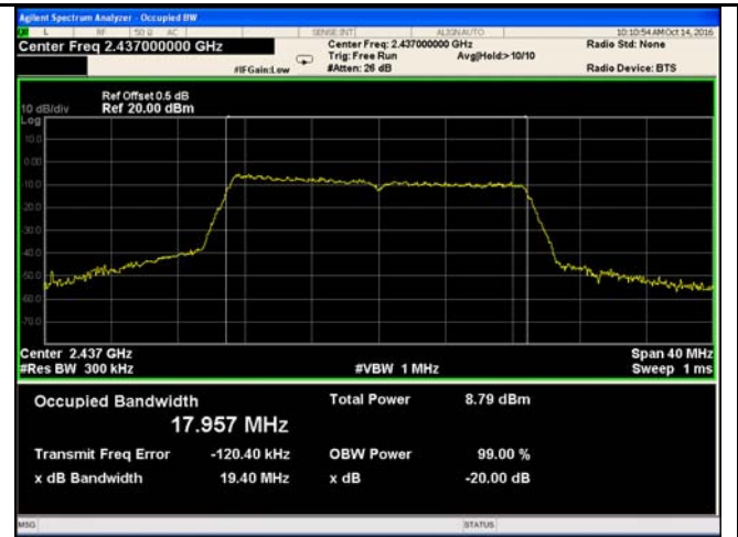
802.11n20 20dB Bandwidth - Mid CH 2437
