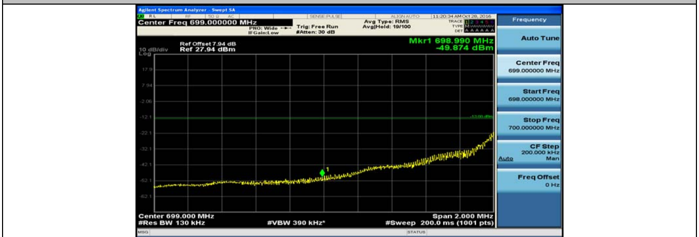
(Channel Bandwidth: 3 MHz)_LCH_16QAM_15RB#0
