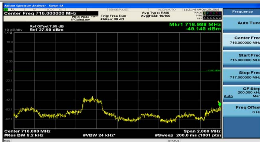
(Channel Bandwidth: 3 MHz)_HCH_QPSK_15RB#0
