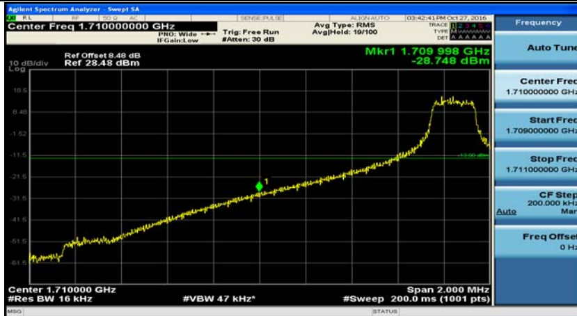
(Channel Bandwidth:15 MHz)_LCH_16QAM_75RB#0
