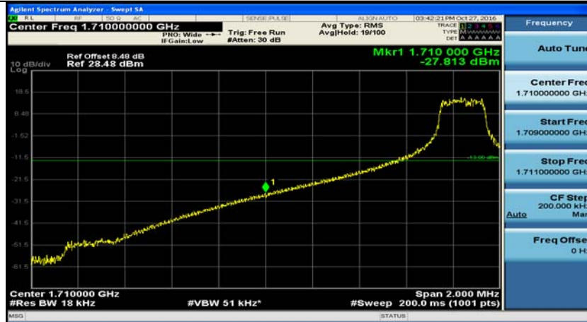
(Channel Bandwidth:15 MHz)_LCH_QPSK_75RB#0
