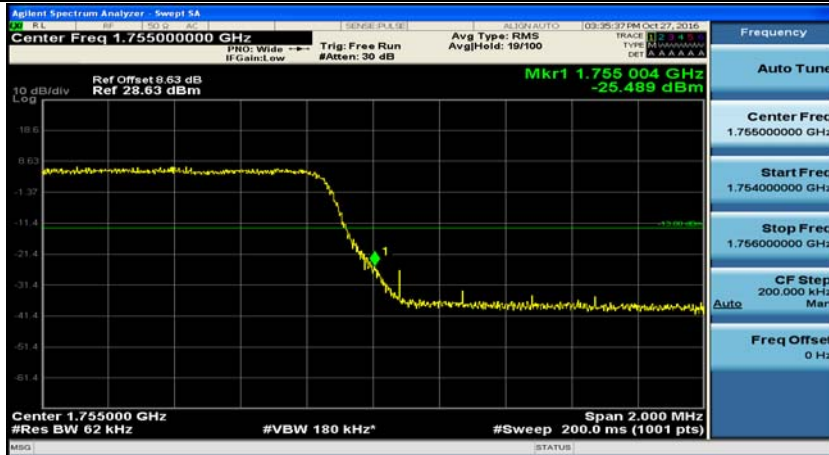
(Channel Bandwidth: 3 MHz)_LCH_16QAM_1RB#0
