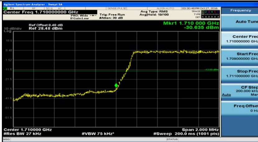
(Channel Bandwidth: 1.4 MHz)_HCH_QPSK_1RB#0
