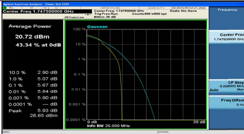
(Channel Bandwidth:15 MHz)_HCH_16QAM_1RB#0
