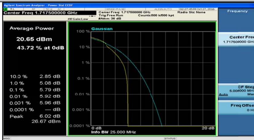
(Channel Bandwidth:15 MHz)_LCH_16QAM_1RB#74
