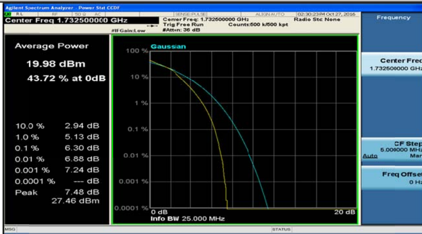
(Channel Bandwidth:15 MHz)_HCH_16QAM_1RB#0
