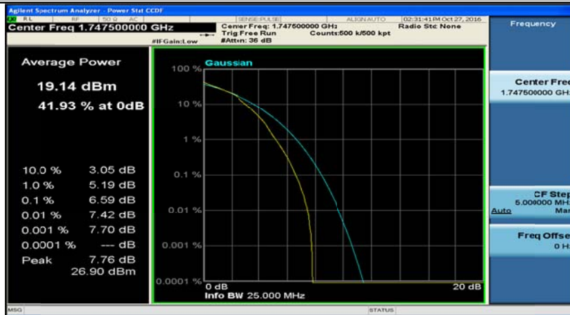
(Channel Bandwidth:15 MHz)_HCH_16QAM_75RB#0
