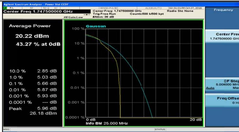
(Channel Bandwidth:15 MHz)_HCH_16QAM_37RB#0
