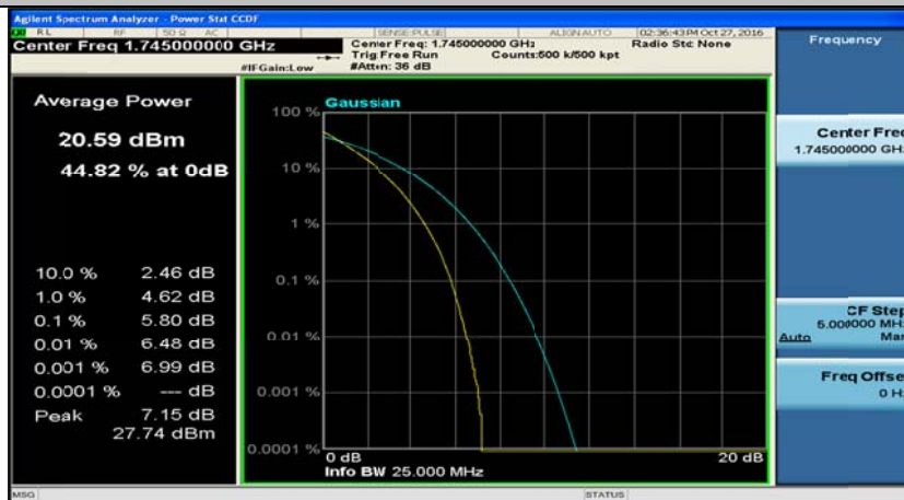
(Channel Bandwidth:20 MHz)_HCH_QPSK_100RB#0
