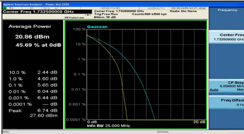
(Channel Bandwidth:15 MHz)_HCH_QPSK_1RB#0
