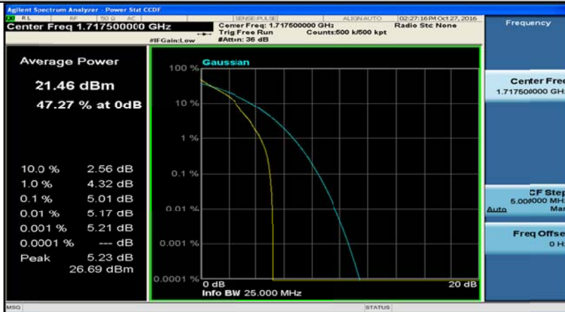
(Channel Bandwidth:15 MHz)_LCH_QPSK_1RB#37
