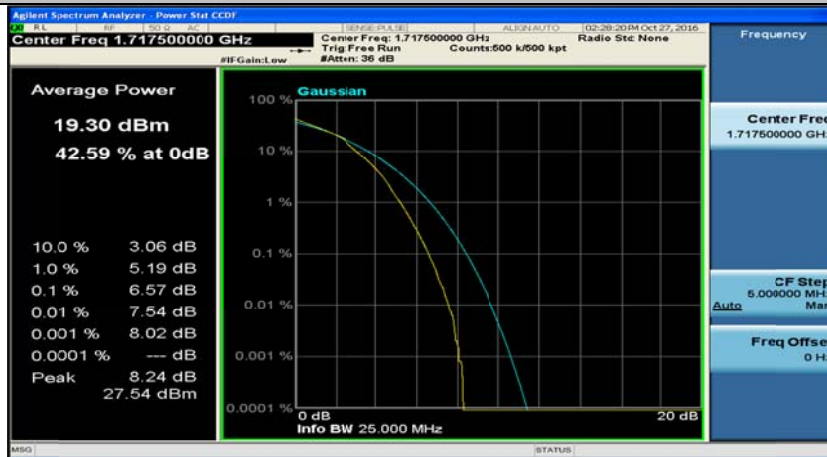
(Channel Bandwidth:15 MHz)_LCH_16QAM_37RB#38
