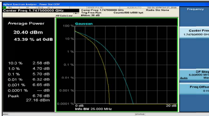
(Channel Bandwidth:15 MHz)_HCH_QPSK_37RB#0
