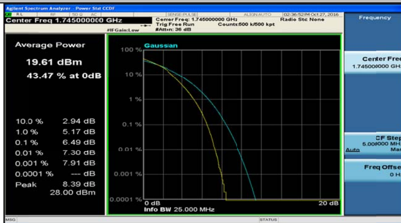
(Channel Bandwidth:20 MHz)_HCH_16QAM_100RB#0
