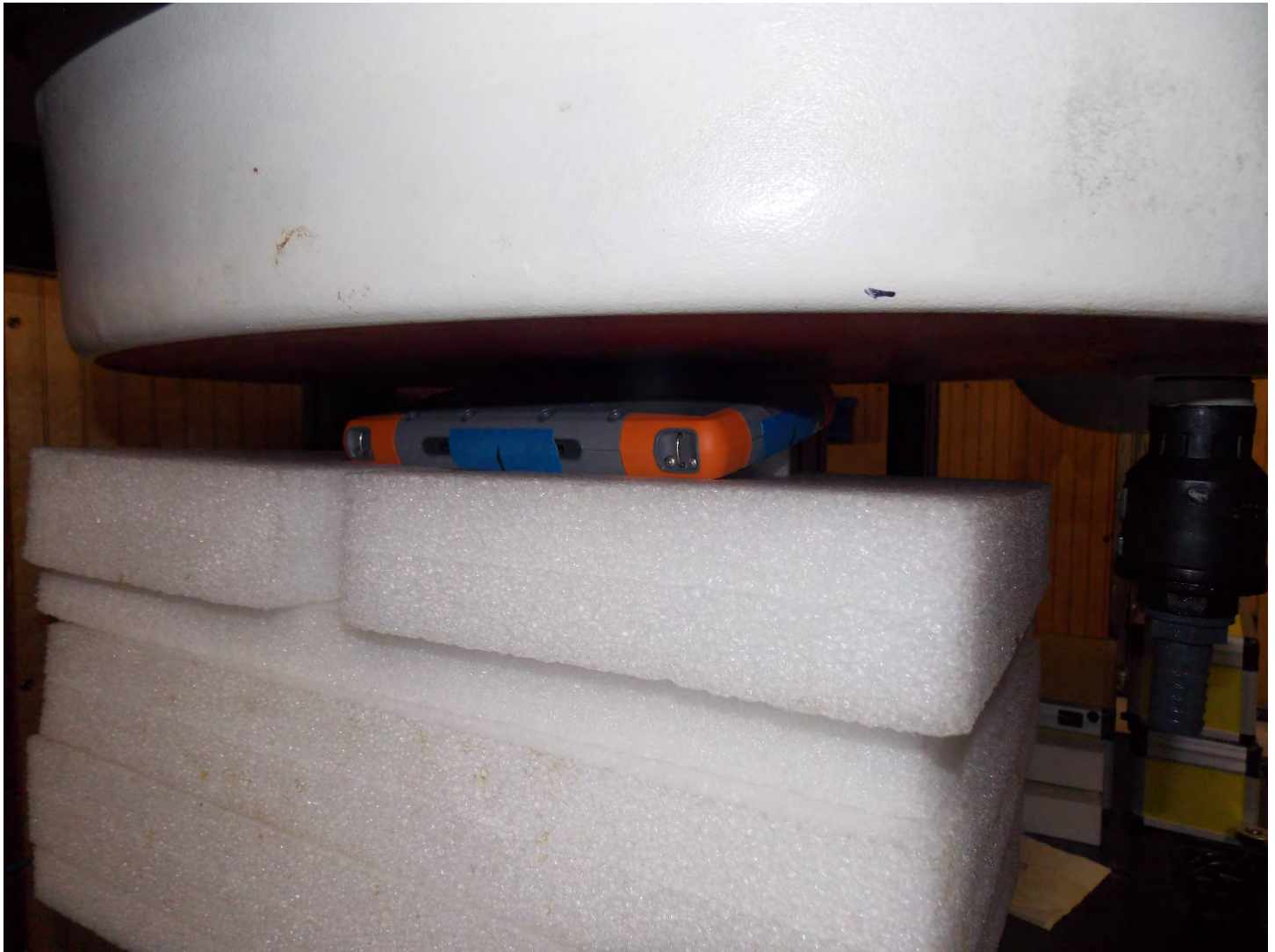
Test Position WWAN Back 0 mm Gap
