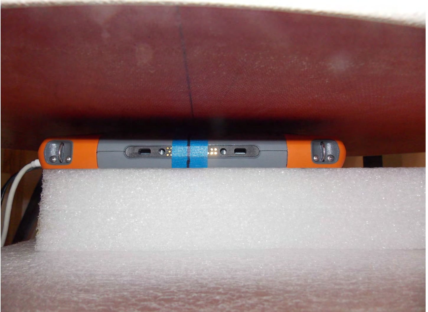
Test Position RFID Back 0 mm Gap
