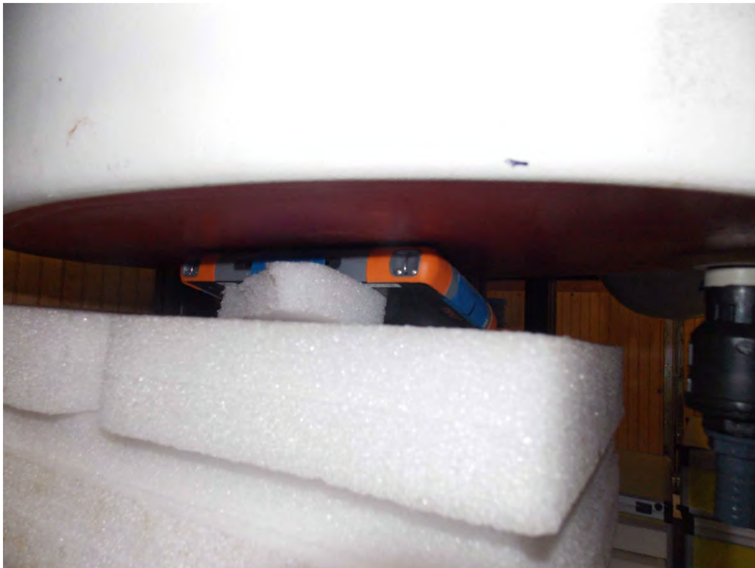
Test Position SAR Back Primary Antenna 0 mm Gap
