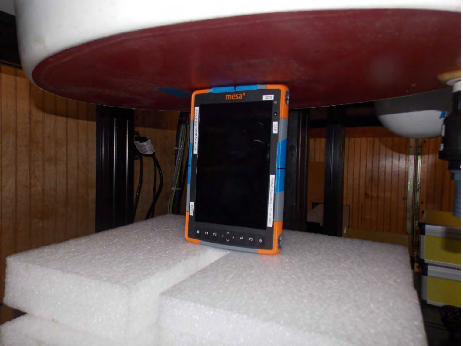
Test Position SAR Top Primary Antenna 0 mm Gap
