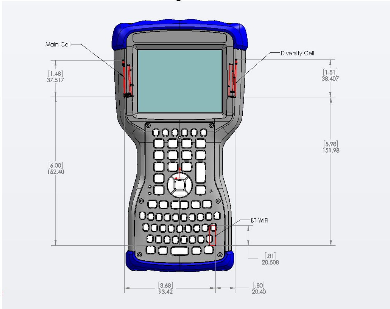
Figure 9.1 SAR Location Diagram of Antenna Distances
