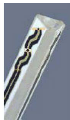
Figure 2.3 Probe Thick-Film Technique
