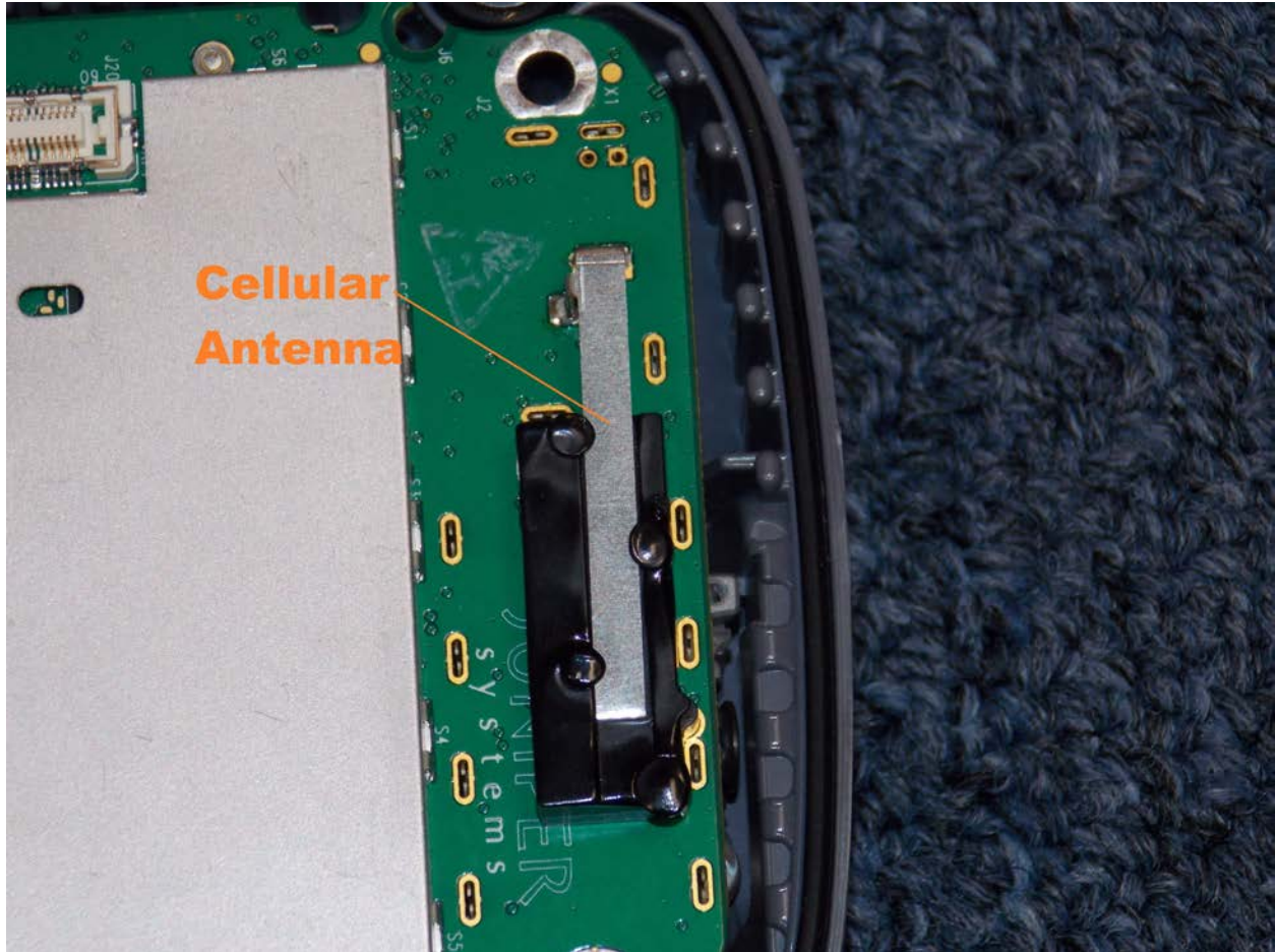
Cellular Antenna Location
