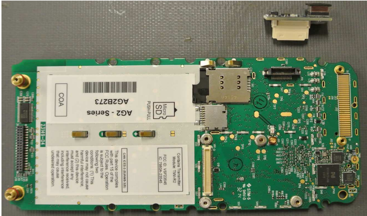
Mainboard bottom with shields removed camera removed
