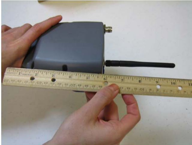
Figure 3: Antenna-to-Hand Separation For Left- and Right-Handed Use (GPS+GSM Pack)
