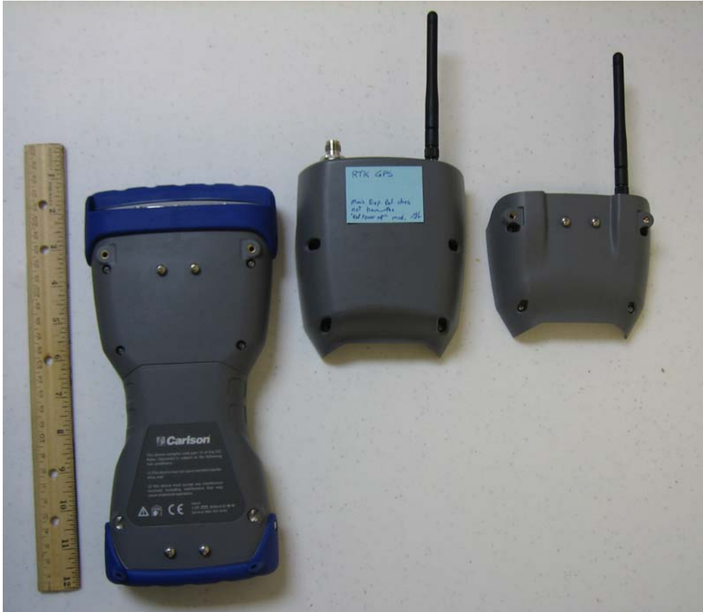
Figure 1: TK6000 and Both Versions of Expansion Pack (GSM+GPS on Left, GSM only on Right)
