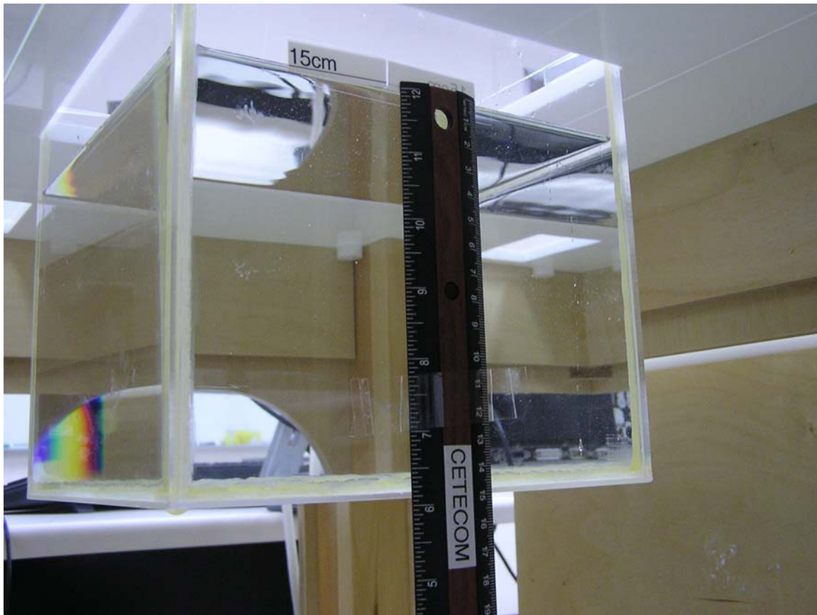
Photo 3. Photo to demonstrate 15 cm Z-axis flat phantom
