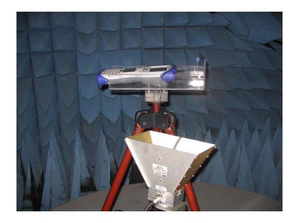
Note – horn antenna in photo is connected to the wireless communications test set to establish the control link to the EUT
