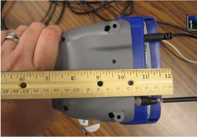
Figure 2: WWAN Antenna-to-Hand Separation For Left- and Right-Handed Use and With Antenna Angled
