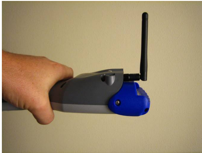
Figure 2: WWAN Antenna-to-Hand Separation For Left- and Right-Handed Use and With Antenna Angled
