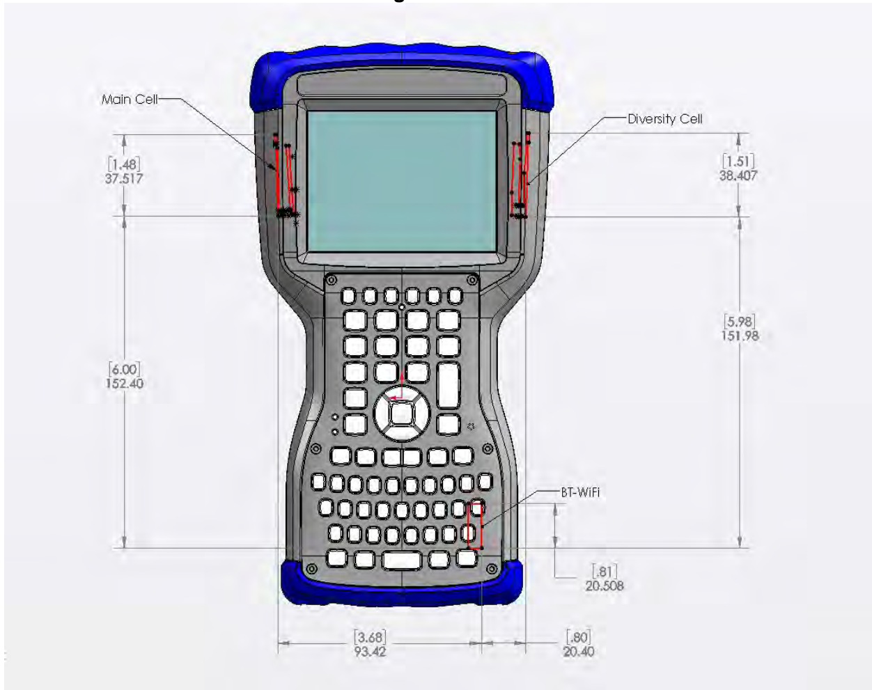
Figure 9.1 SAR Location Diagram of Antenna Distances
