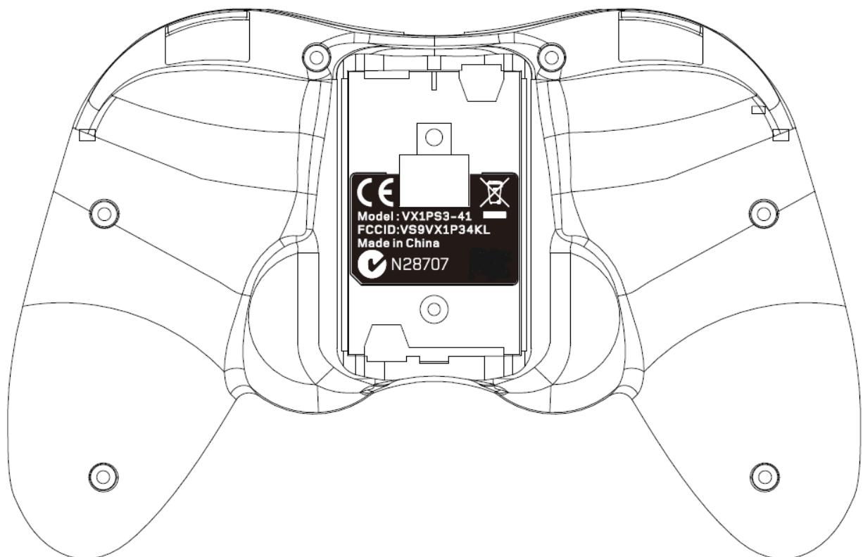
The ID label is in the battery compartment, we will market the device without the battery installed.
