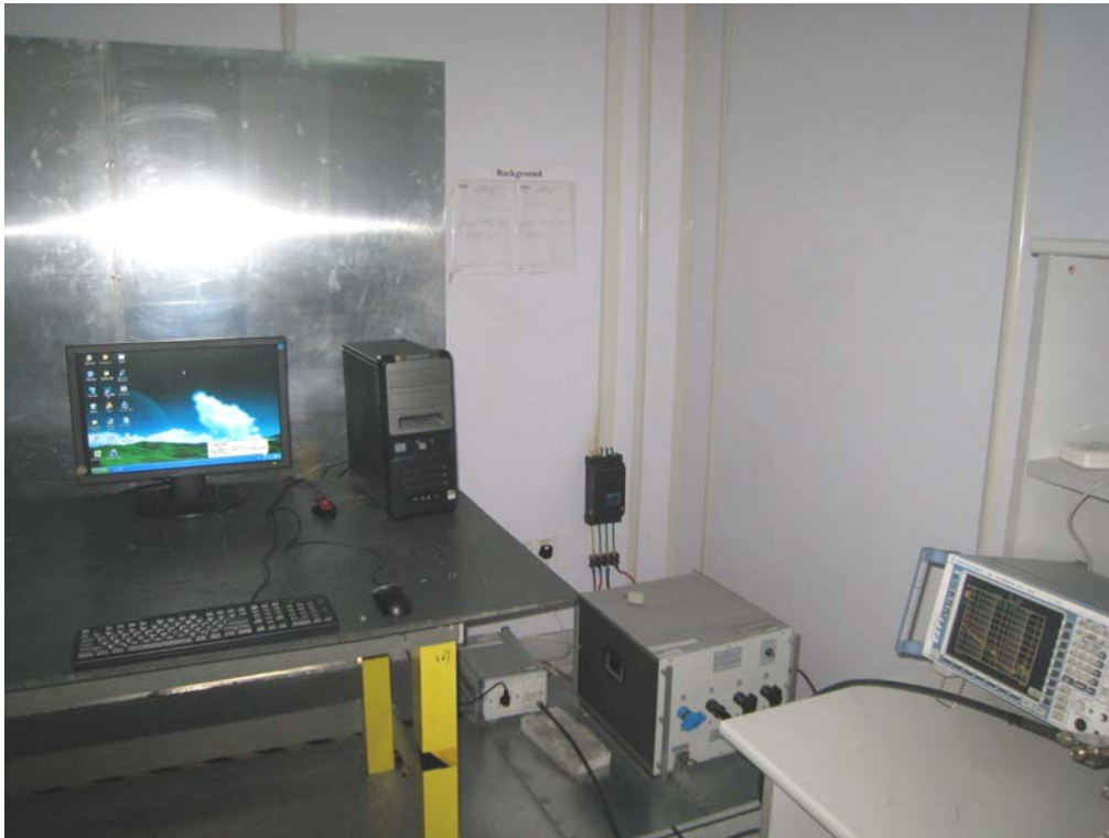
Line Conducted Emission Test Setup
