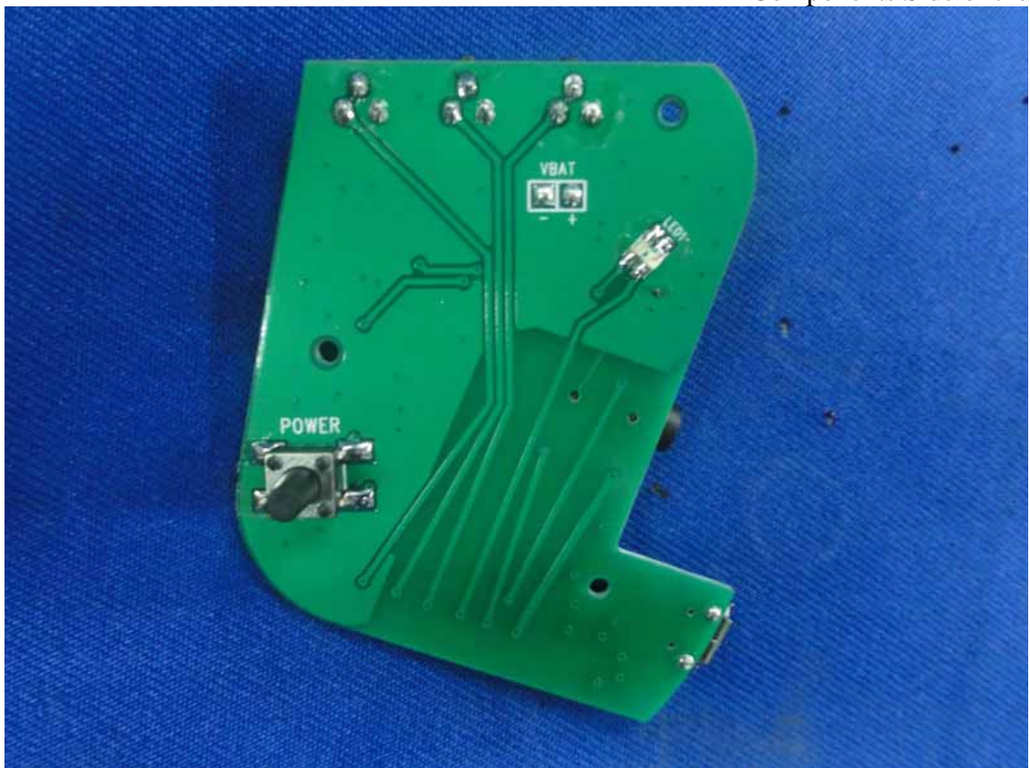
Figure 22 Components Side of the PCB
