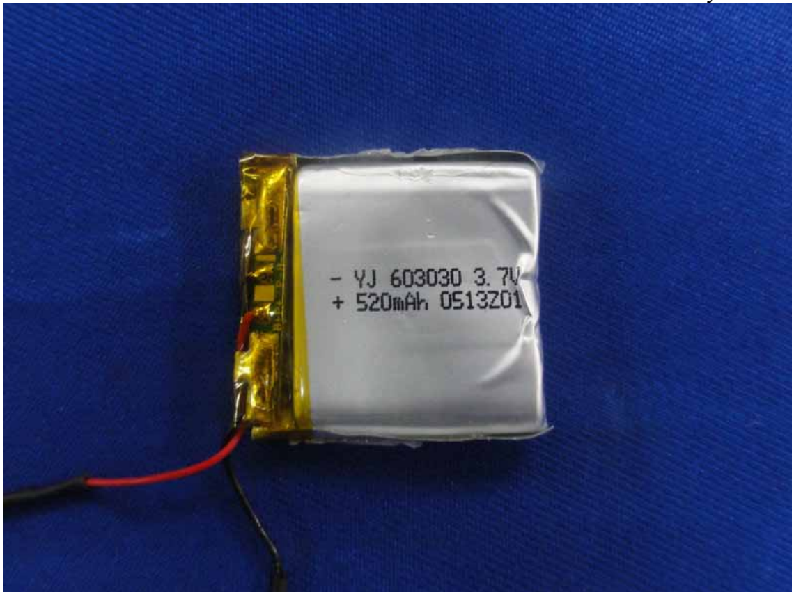
Figure 23 Battery of the EUT
