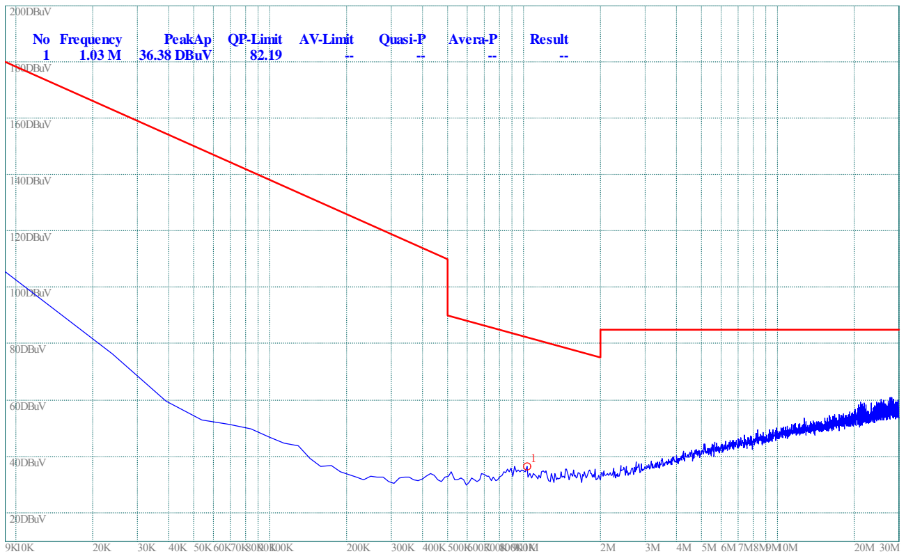
(Plot A.0: 9kHz to 30MHz @ GFSK, channel 3)
