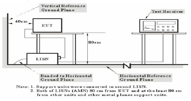
The setup of EUT is according with MP-5 measurement procedure. The specification used was the FCC Part 18 limits.
