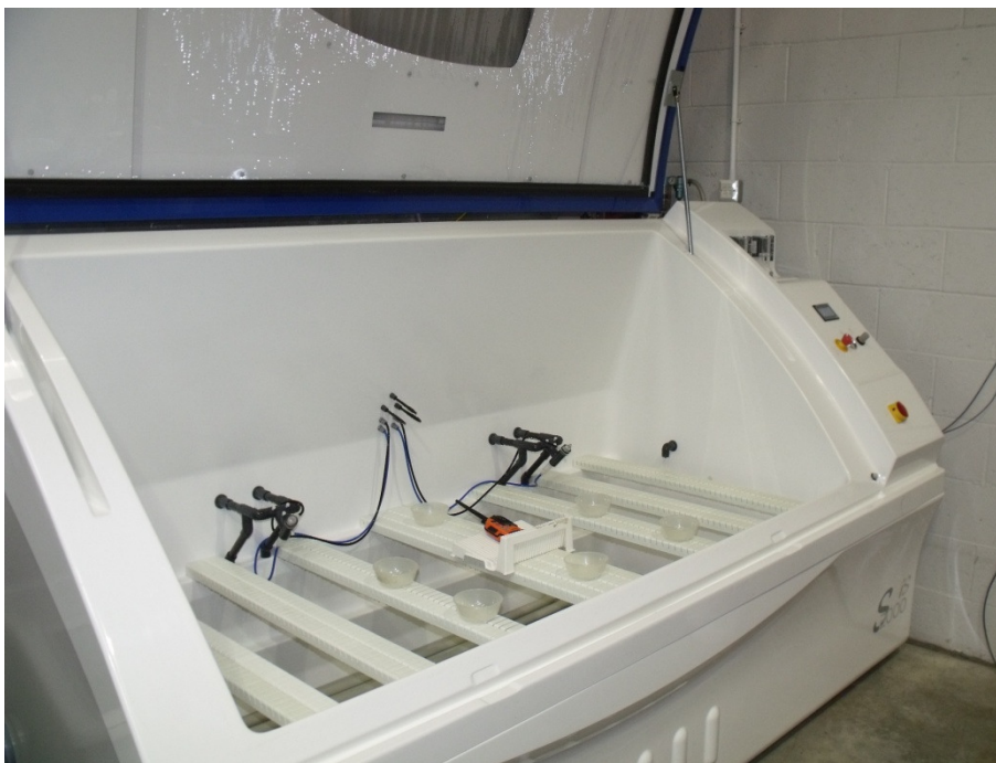
Test Setup Photo – Salt Spray Chamber
