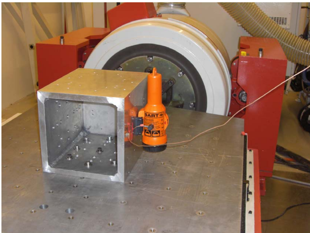
Picture 3: Shows the EUT during vibration in x axis
