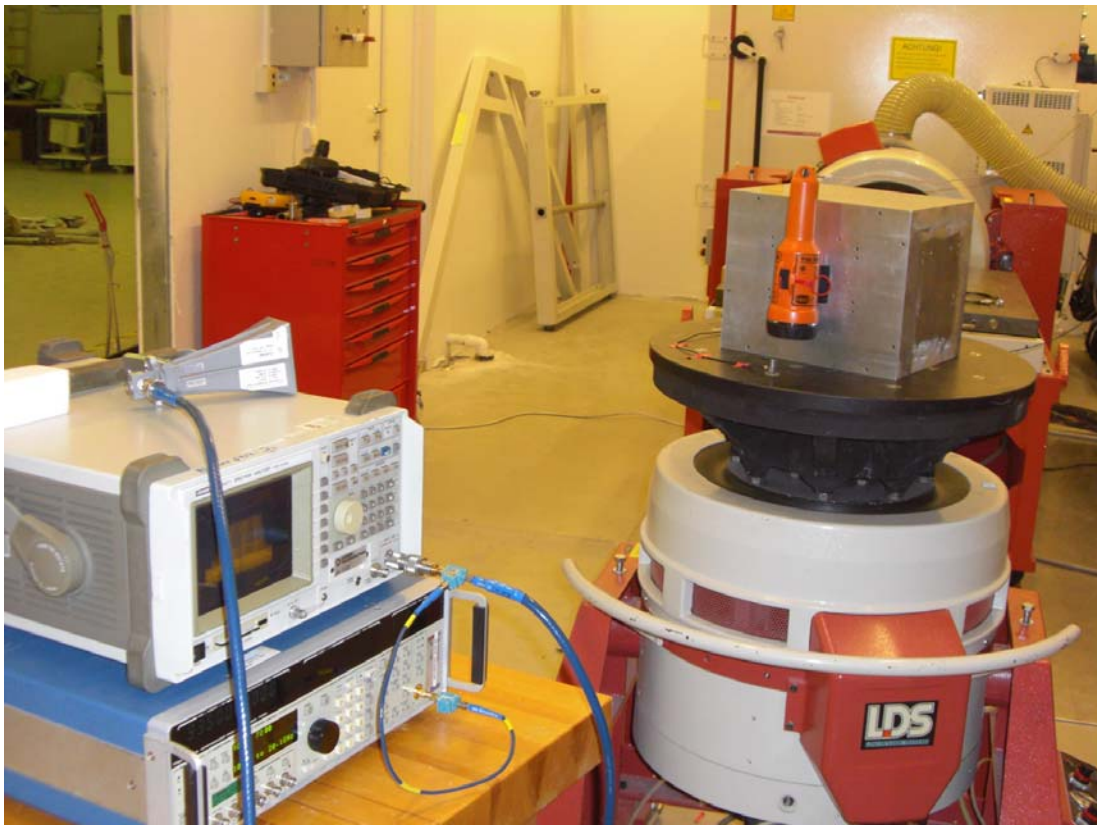
Picture 5: Shows the EUT during vibration in z axis
