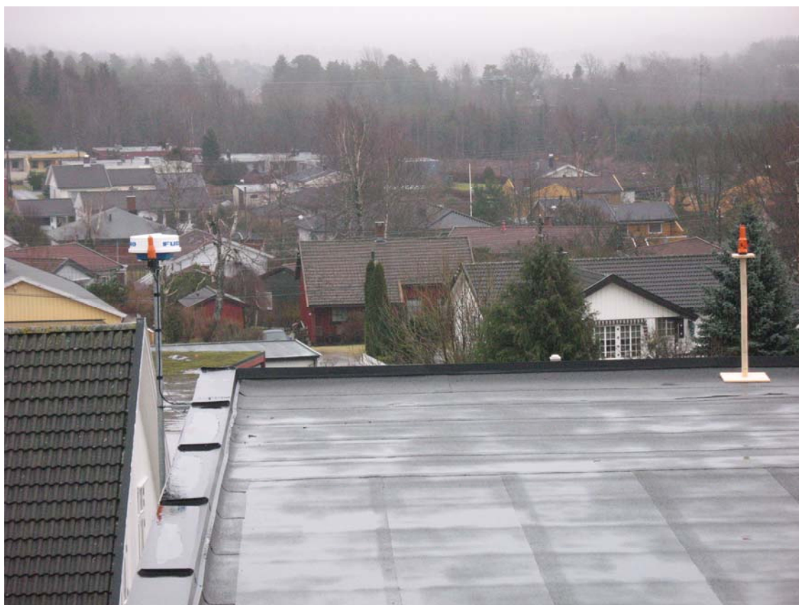
Picture 2: Shows EUT (to the right) and radar (to the left) during receiver front end protection test
