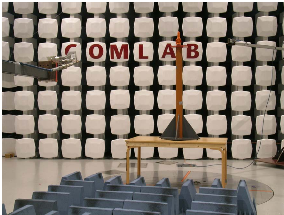
Picture 1: Shows the measurement setup during “Antenna characteristics” measurements. The EUT is positioned on a pedestal 2,2 meters above ground level and the floor between EUT and measurement antenna is covered with absorbers to eliminate ground reflections.
