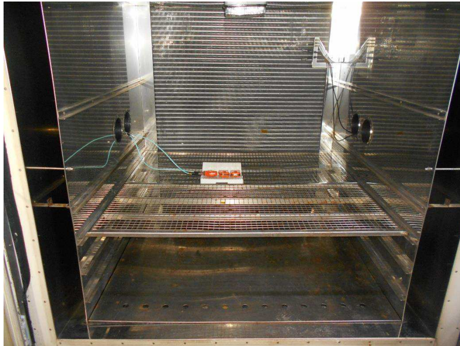
Figure 2 - Dry Heat Functional test setup – EUTs close-up and installed in climatic chamber
