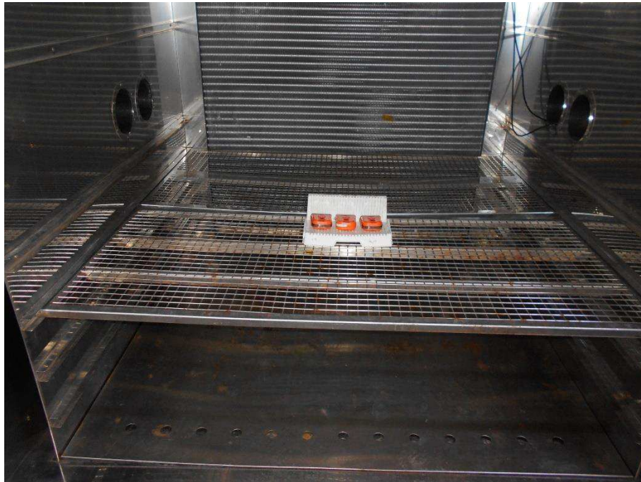
Figure 7 – Low Temperature Storage test setup – EUTs close-up and installed in climatic chamber
