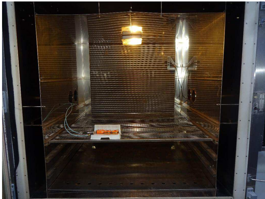
Figure 6 - Damp Heat test setup – EUTs close-up and installed in climatic chamber
