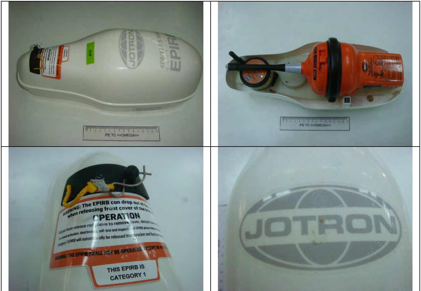
Figure 6.3 – View exterior inspection of the EUT upon completion of the salt fog test
