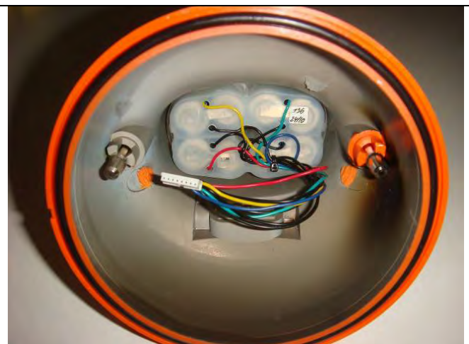
Figure 8.8 – Detailed examination of EPIRB Tron 60GPS upon completion of the drop test. There is no water inside.
