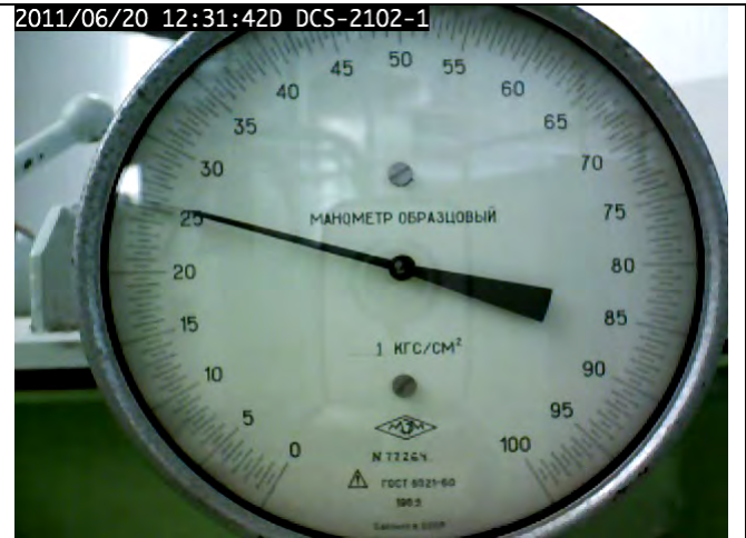
Figure 15.14 – Pressure meter at the moment of activation
