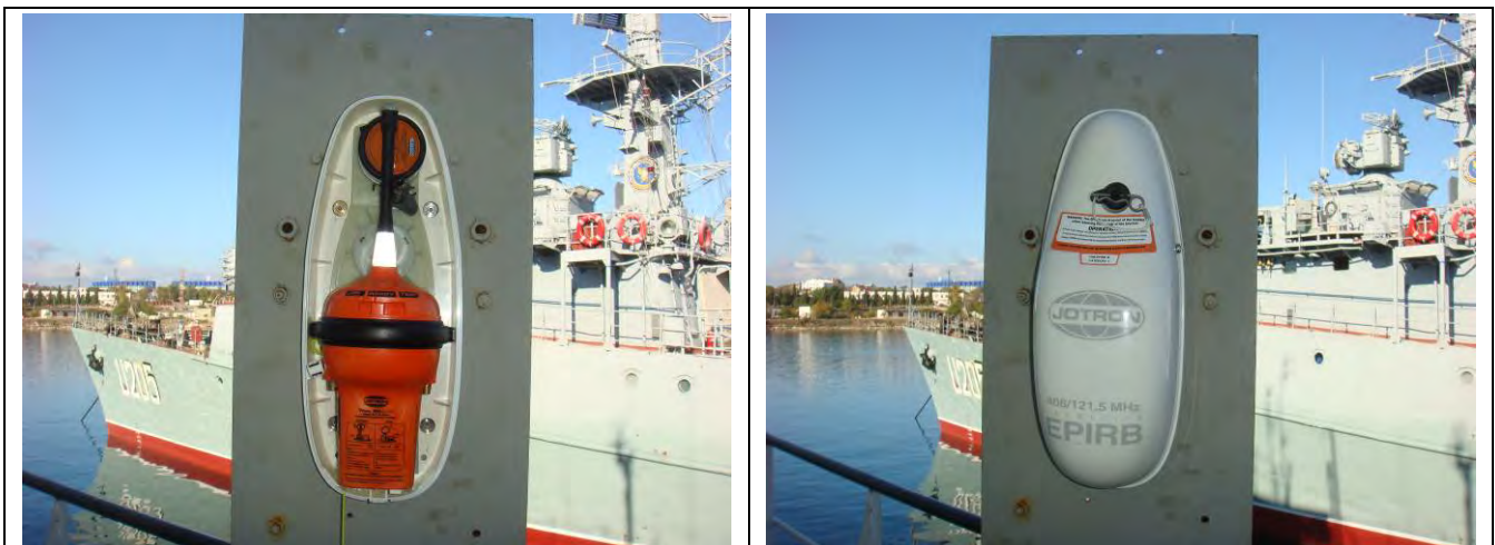
Figure 13.1 – EUT (EPIRB and release mechanism) mounted on the rotatable support before test.
