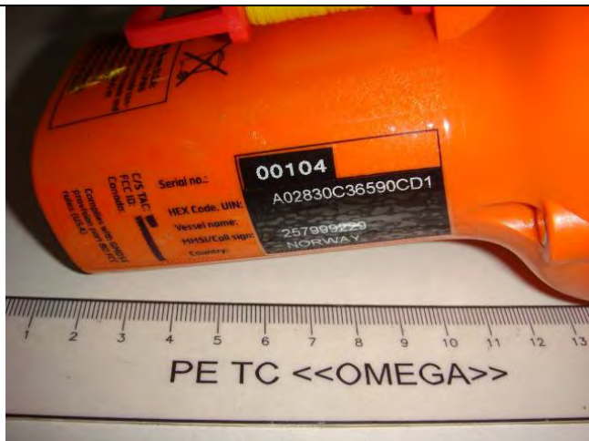
Figure 8.6 – Detailed examination of EPIRB Tron 60GPS upon completion of the drop test. There is no water inside.
