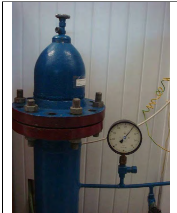
Figure 9.1 – View of immersion test site (Manometer of immersion test site indicates 1 bar)
