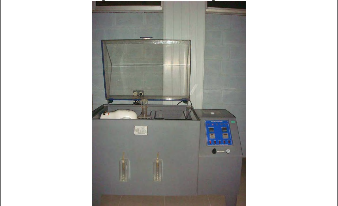
Figure 6.2 – View of the EUT in salt fog chamber
