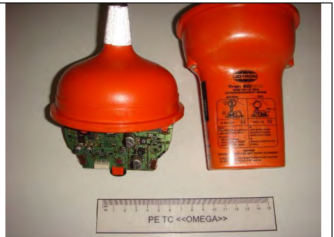
Figure 8.7 – Detailed examination of EUT upon completion of the drop test. There is no water inside.
