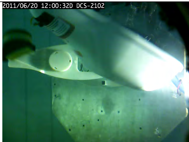
Figure 15.9 – View of automatic release mechanism in rolling 90° starboard position at the moment of activation
