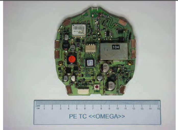
Figure 19.4 – View of the PCB (EPIRB Tron 60GPS) upon completion of the humidity test
