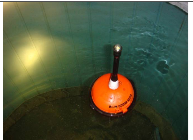
Figure 15.12 – Emersion after released in rolling 90° port position
