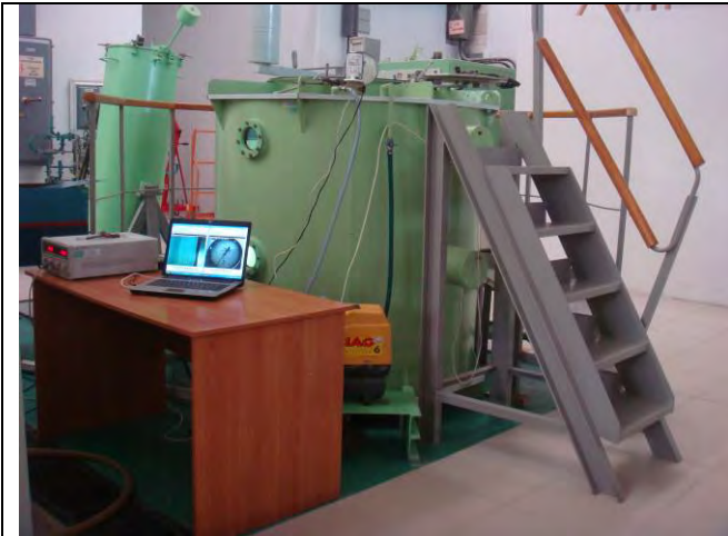
Figure 15.1 - Total view of hydrostatic tank
