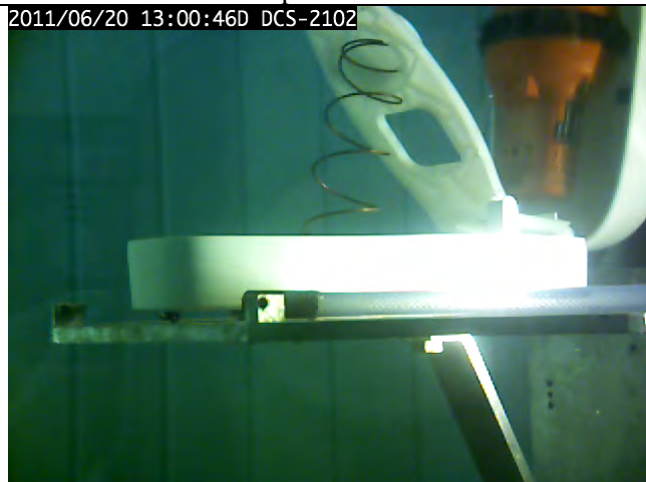
Figure 15.21 – View of automatic release mechanism in rolling 90° stern down position at the moment of activation
