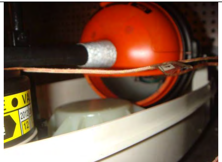
Figure 19.2 - View of the modified EPIRB installed in release mechanism
