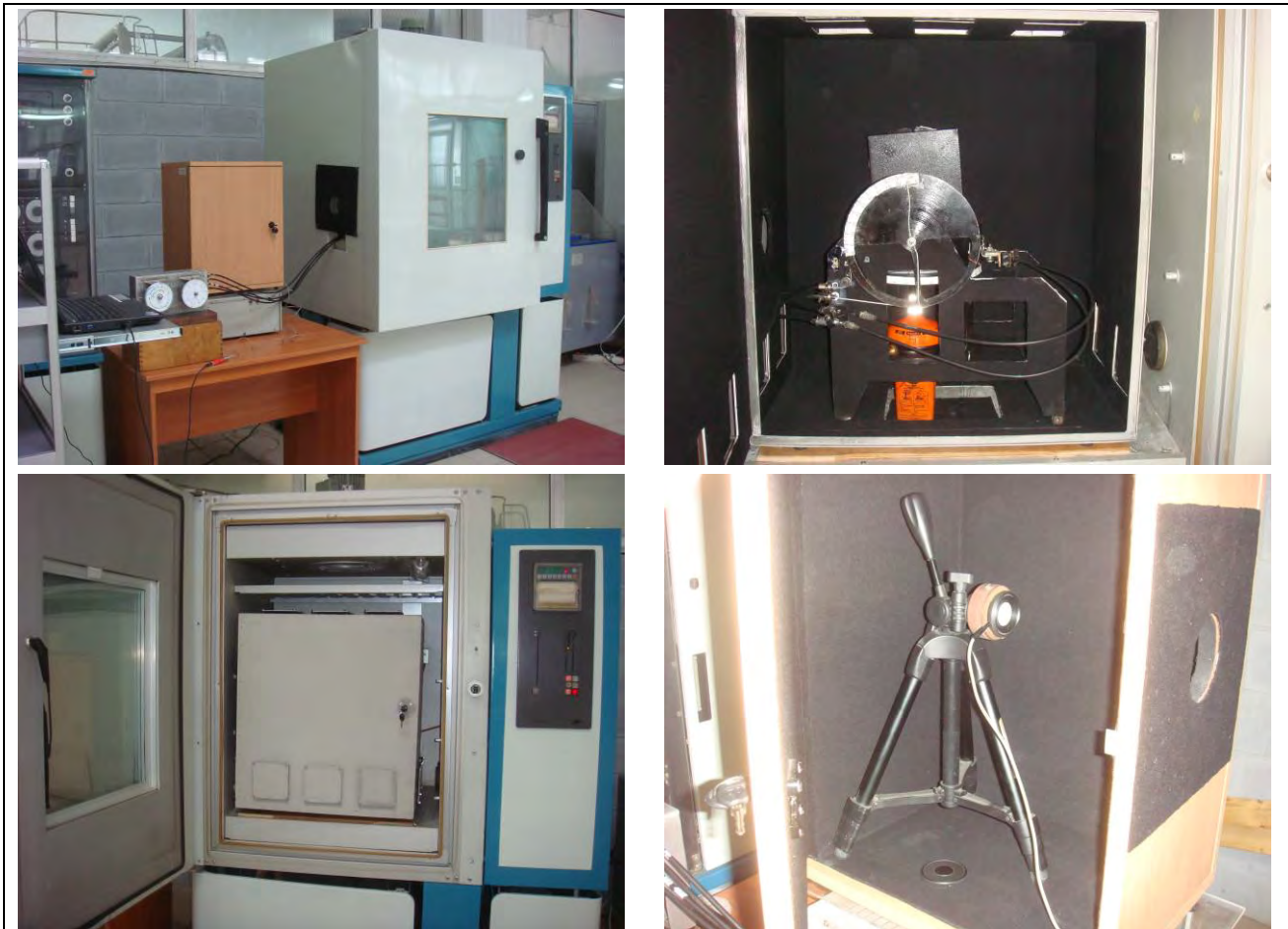
Figure 13.1 – Low-duty cycle light test. The EPIRB Tron 60GPS stays in the climatic chamber. General view of test equipment for low-duty cycle light test
