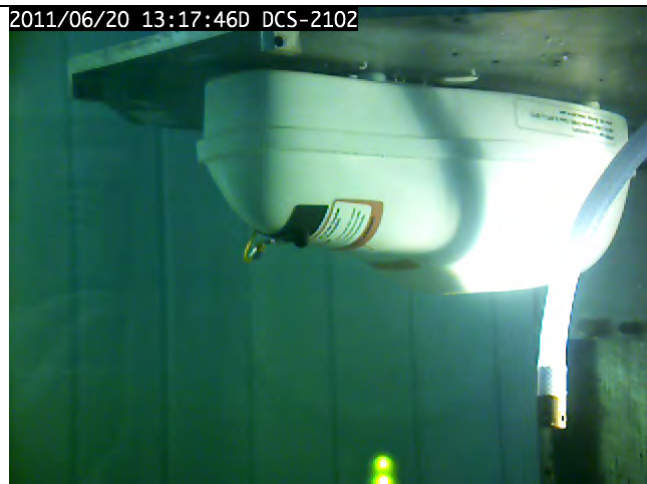
Figure 15.15 – Immersion in rolling 90° bow down position before activation test
