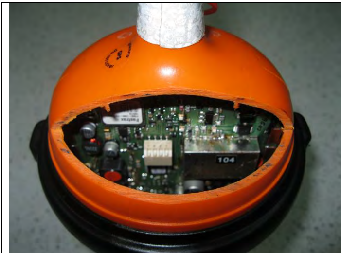
Figure 19.1 - View of the EPIRB Tron 60GPS with the modified housing before the humidity test
