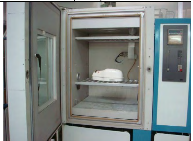
Figure 3.3 – View of the EPIRB Tron 60GPS before damp heat cycle in chamber
