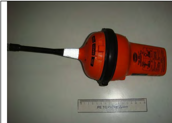
Figure 8.1 – View EPIRB Tron 60GPS before of the drop test in water
