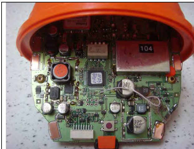
Figure 9.2 – The PCB after immersion test. There is no water ingress.
