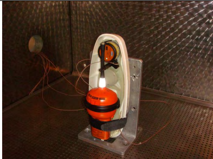
Figure 19.3 - View of the modified EPIRB in release mechanism in climatic chamber
