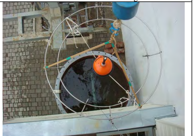
Figure 8.4 – View EPIRB Tron 60GPS dropping in water with antenna vertical up
