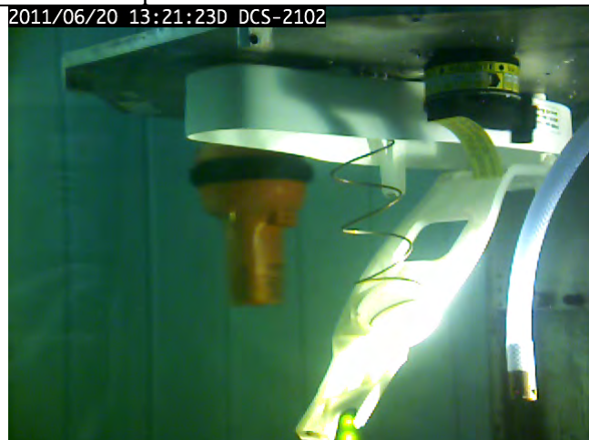
Figure 15.17 – View of automatic release mechanism in rolling 90° bow down position at the moment of activation
