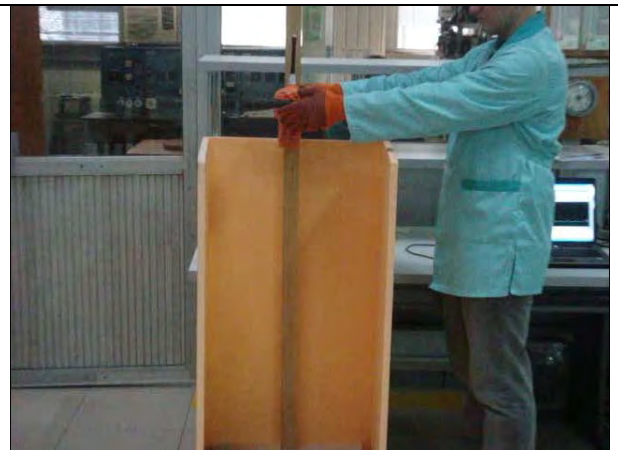
Figure 7.7 – View the orientation of the Tron 60GPS before of the drop test
