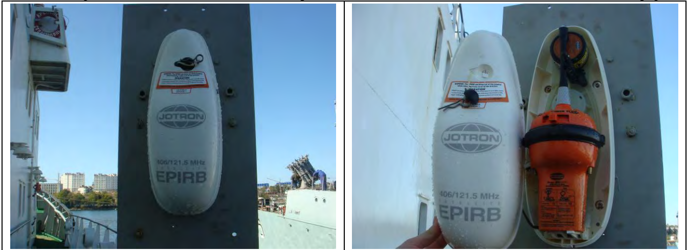
Figure 13.3 - View of EUT upon completion of inadvertent activation test
