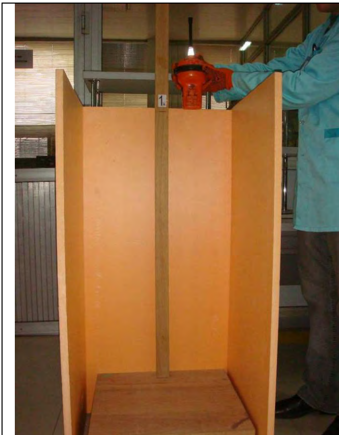
Figure 7.4 – Total view of test site of the drop from a height of 1 m above the test surface
