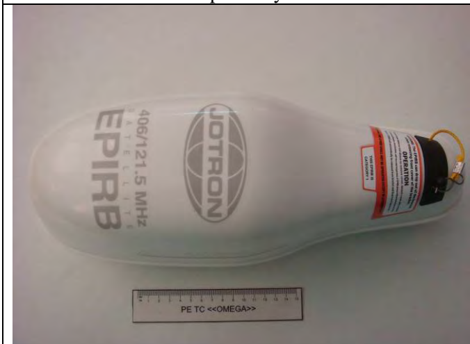
Figure 3.4 – Results of EPIRB Tron 60GPS at the end of the 2 hour period in the +40 °C and 93 % relative humidity chamber
