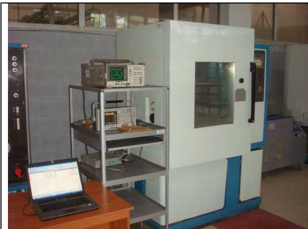
Figure 18.2 – Site for Carrier Frequency Test and Modulation Characteristic Measurement at the minimum, ambient and maximum operating temperatures
