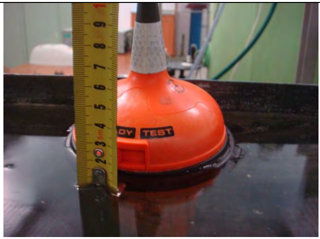
Figure 16.2 – Measuring of distance from water level to the base of antenna while EUT floating in calm fresh water.
