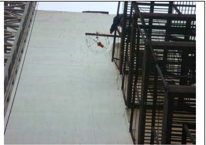
Figure 8.2 – Total view of test site of the drop test in water of EPIRB Tron 60GPS from a height of 20 m
