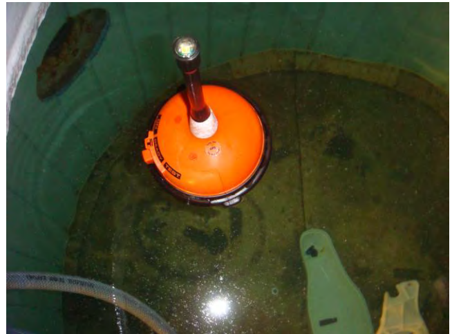
Figure 18.28 – EPIRB emersion after immersion in the normal mounting position after exposure -30 °C
