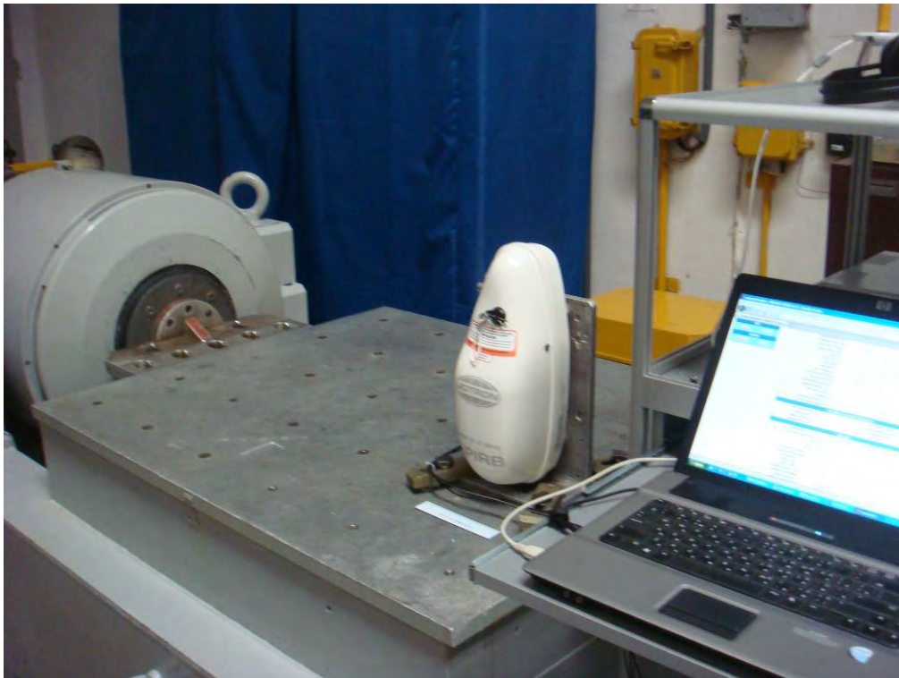
Figure 4.5 - Vibration test in horizontal axis Y
