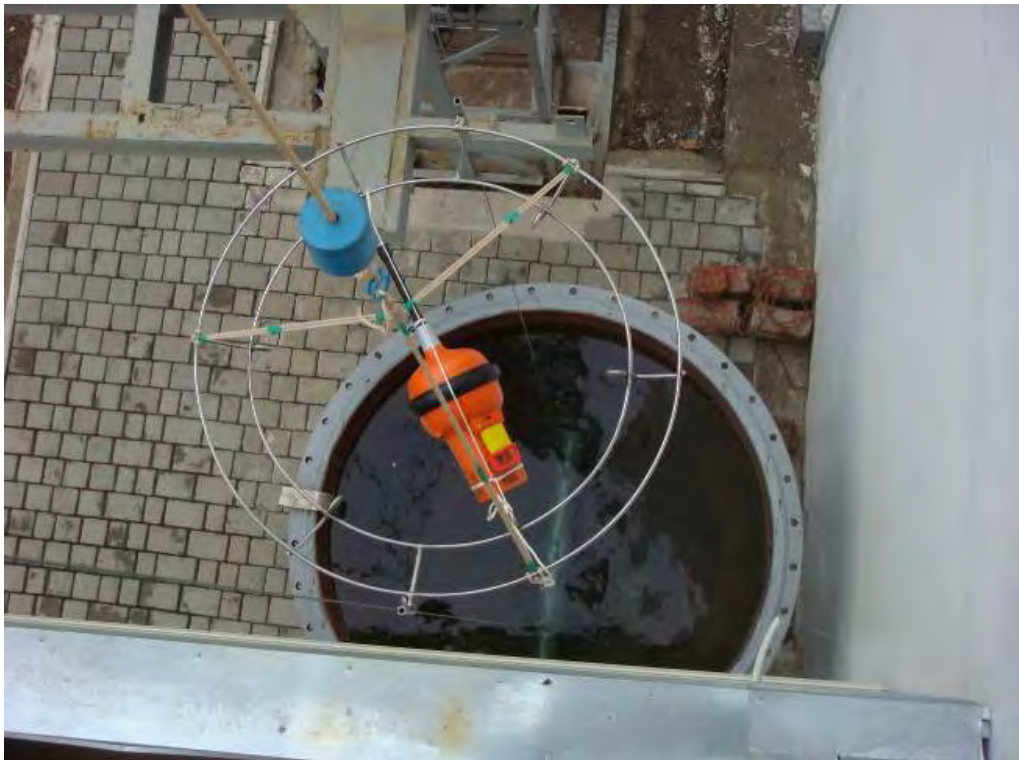
Figure 6.2.3 - EUT dropping in water with antenna horizontal.
