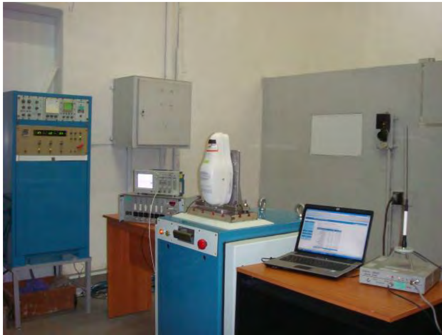
Figure 5.1 - EUT set-up for ruggedness test
