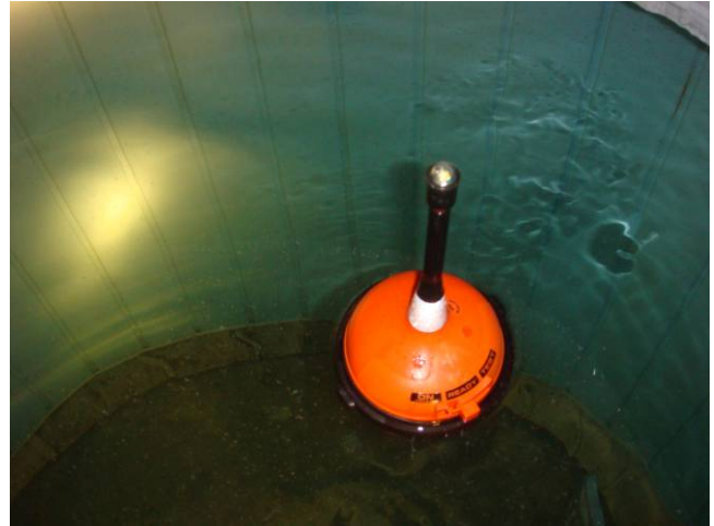
Figure 18.16 – EPIRB floating after immersion in the rolling 90° to port position
