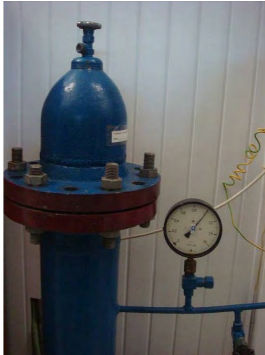
Figure 8. 1 - Hydraulic pressure set-up (1 bar)
