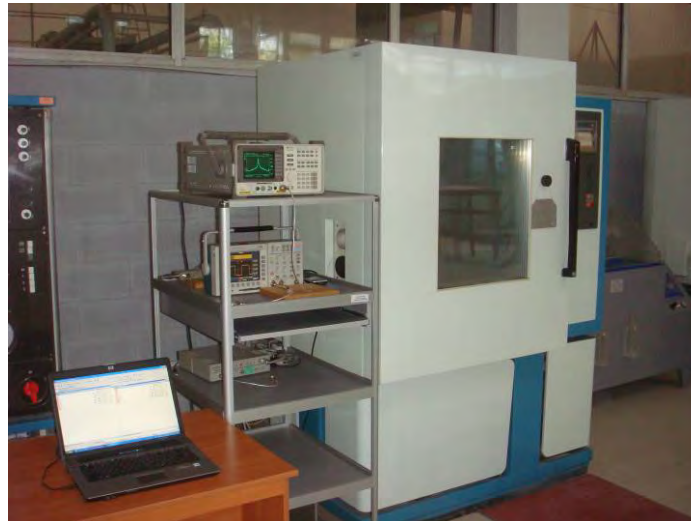
Figure 10.1 – View of the test setup for the Spurious Emissions Test
