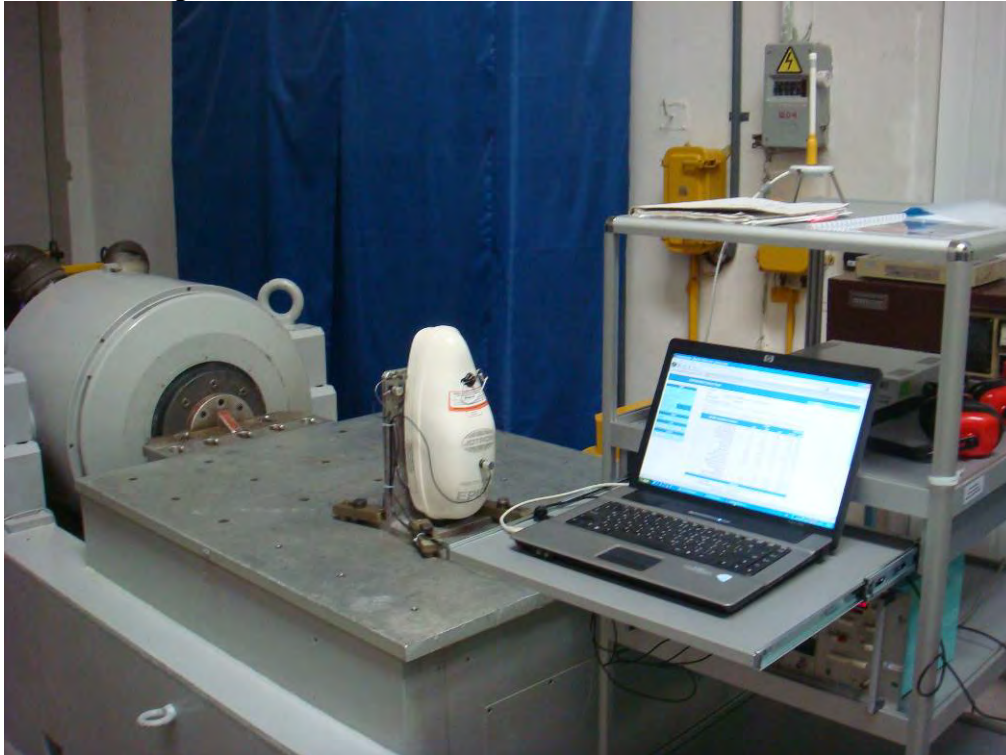
Figure 4.3 - Vibration test in horizontal axis X
