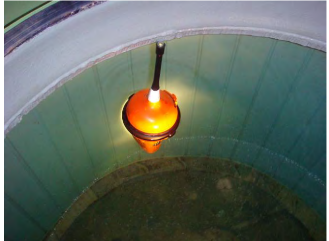
Figure 18.12 – EPIRB floating after immersion in the rolling 90° to starboard position
