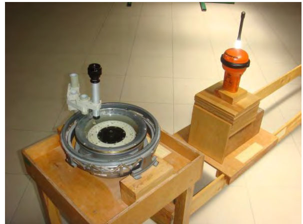
Figure 17.2 – Changing the position EPIRB Tron60GPS around the horizontal and vertical axis. Maximum deviation search.
