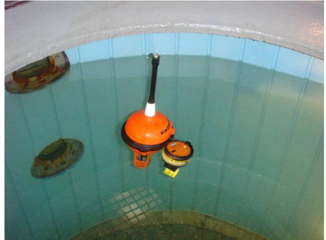
Figure 18.24 – emersion after immersion in the pitching 90° stern down position
