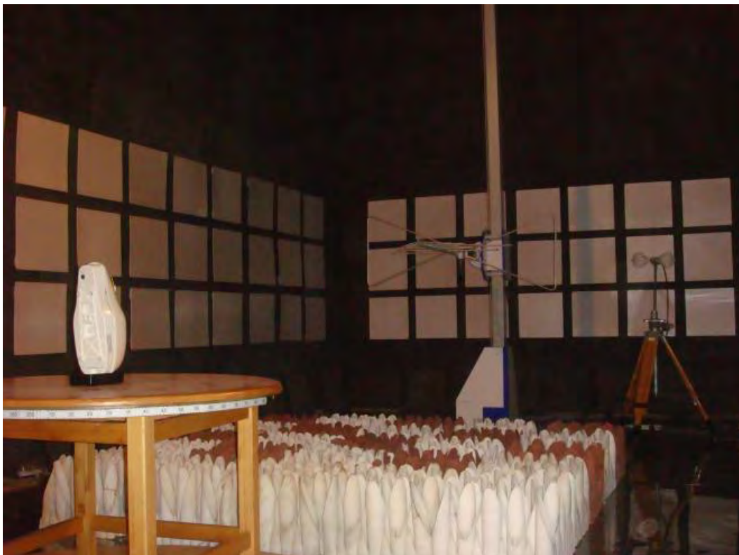
Figure 11. 3 - General view of immunity test set-up. Horizontal polarization.
