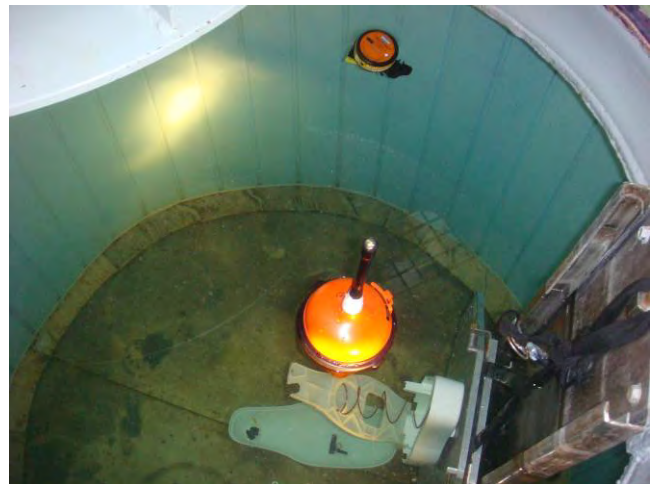
Figure 18.32 – Emersion after immersion in the normal mounting position after exposure at temperature +70 °C
