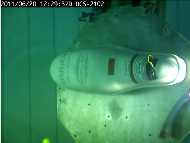
Figure 18.15 – Immersion in the rolling 90° to port position
