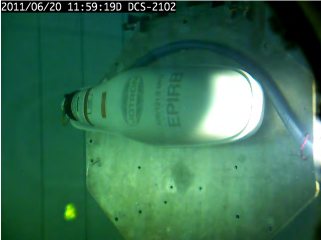
Figure 18.11 – Immersion in the rolling 90° to starboard position
