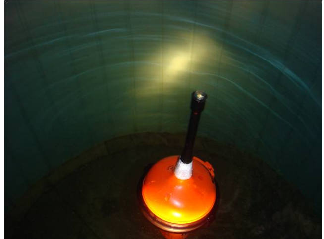
Figure 18.20 – EPIRB floating after immersion in the pitching 90° bow down position
