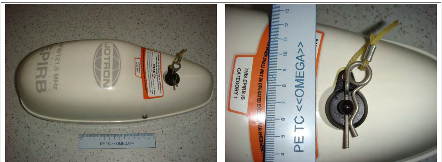
Figure 15.2 - EUT after oil resistance test
