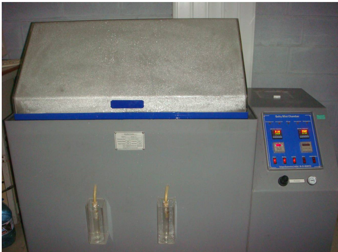
Figure 19.4 – View of EUT in salt fog chamber
