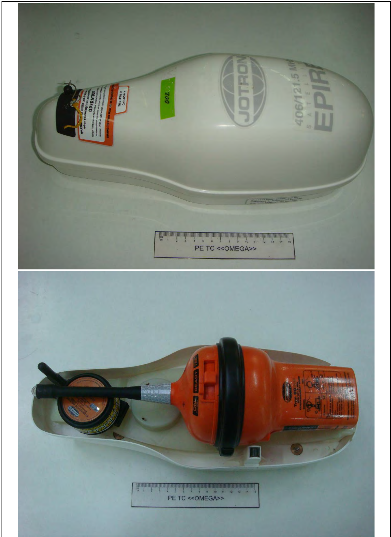
Figure 19.5 - View exterior inspection of EUT upon completion of the salt fog test
