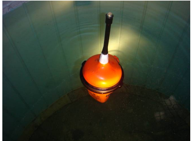
Figure 18.8 – EPIRB floating after immersion in the upside-down position
