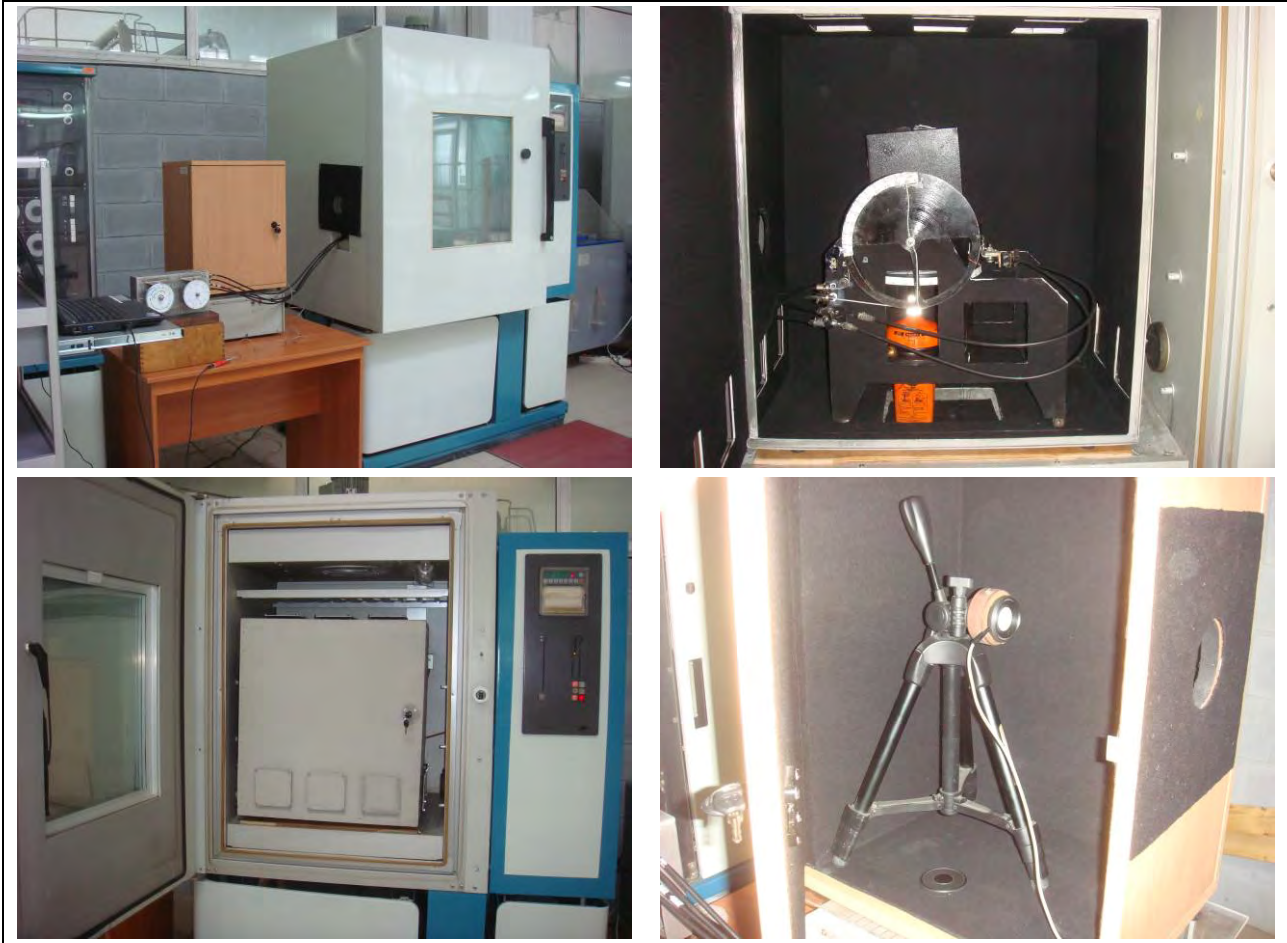
Figure 20.1 – Low-duty cycle light test. The EPIRB Tron 60GPS stays in the climatic chamber. General view of test equipment for low-duty cycle light test
