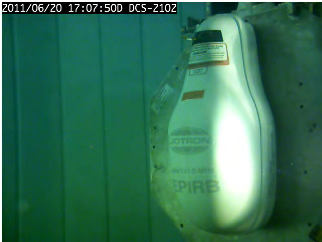
Figure 18.27 – Immersion in the normal mounting position after exposure of EPIRB at minimum temperature -30 °C
