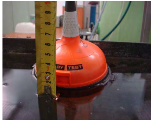
Figure 16.2 – Measuring of distance from water level to the base of antenna while EUT floating in calm fresh water.
