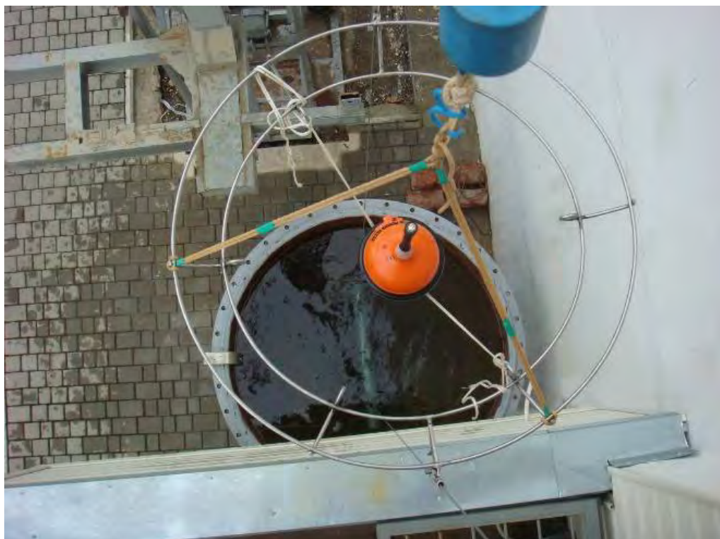
Figure 6.2.2 - EUT dropping in water with antenna vertically up.
