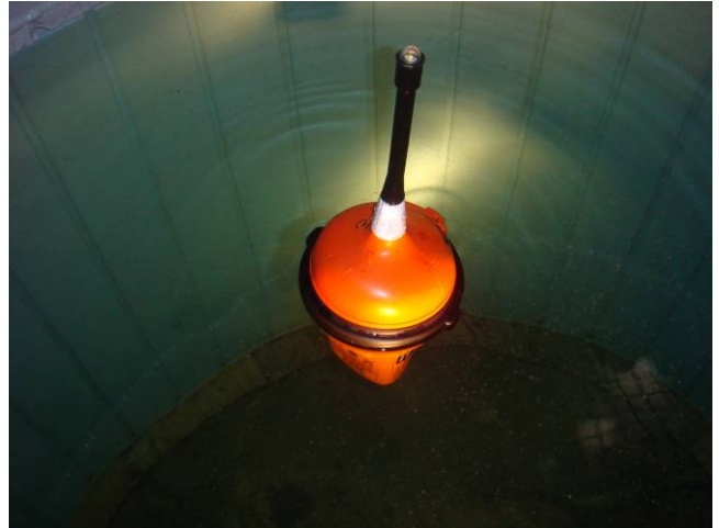
Figure 18.4 – EPIRB floated after immersion in the normal mounting position
