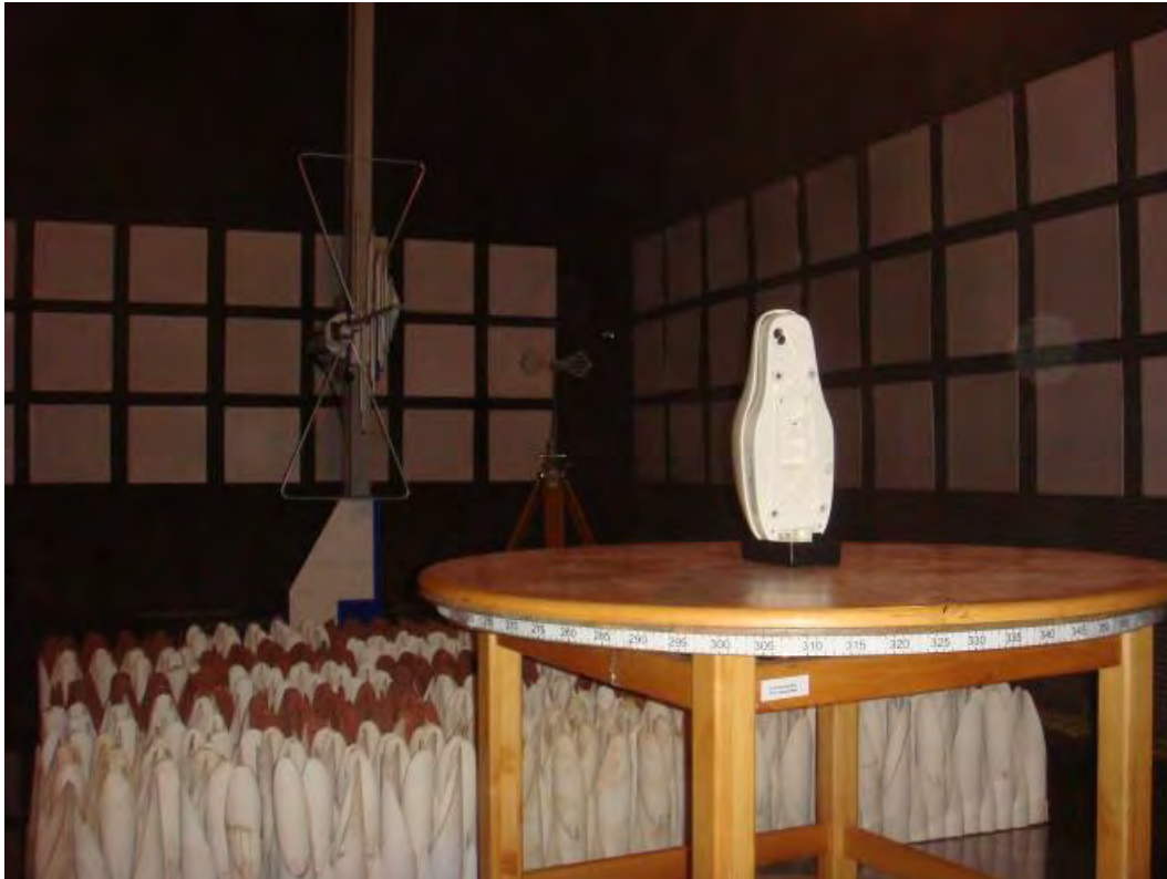
Figure 11. 2 - General view of immunity test set-up. Vertical polarization.
