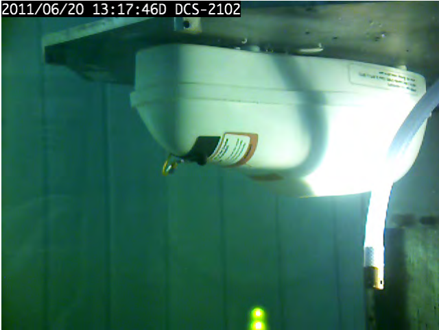
Figure 18.19 – Immersion in the pitching 90° bow down position
