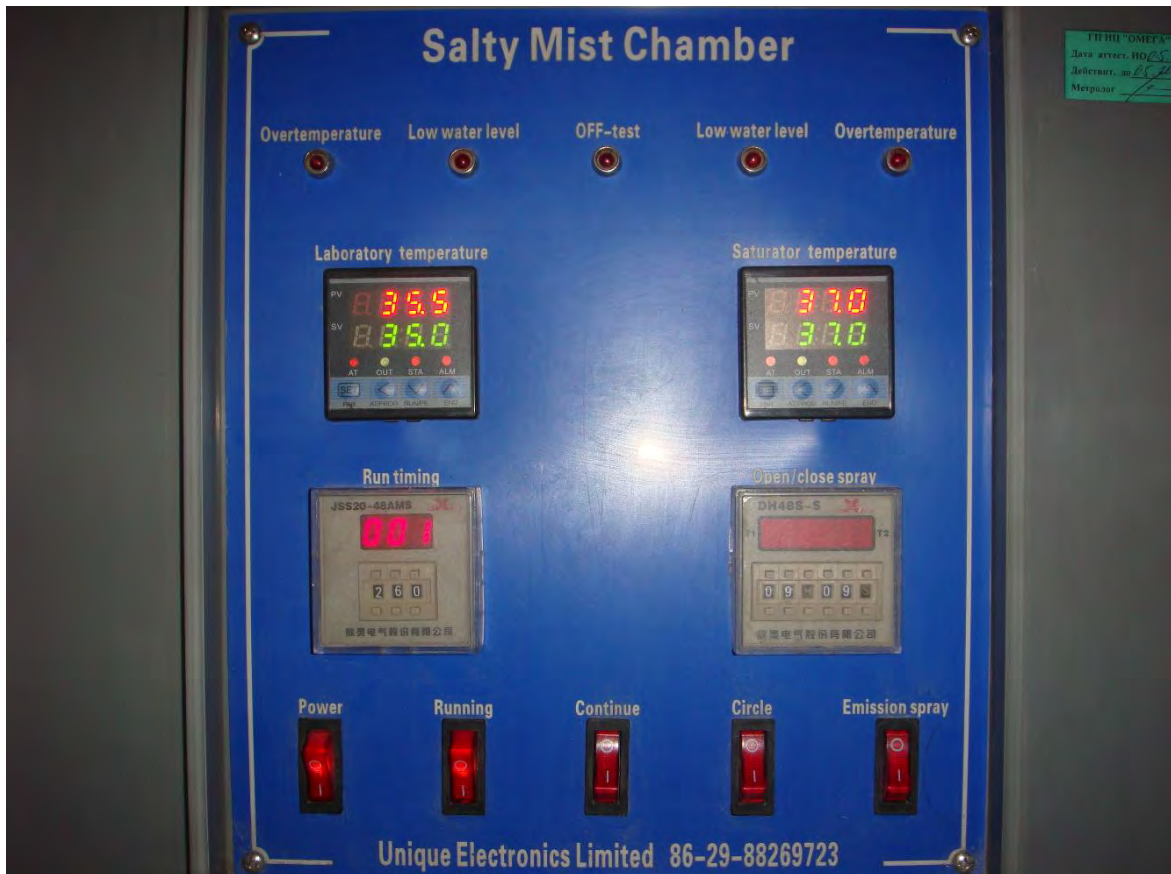
Figure 19.3 – Temperature setup of salt solution
