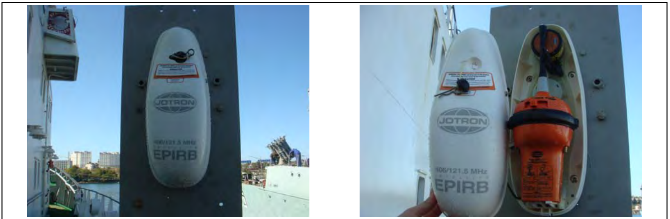
Figure 13.3 - View of EUT upon completion of inadvertent activation test
