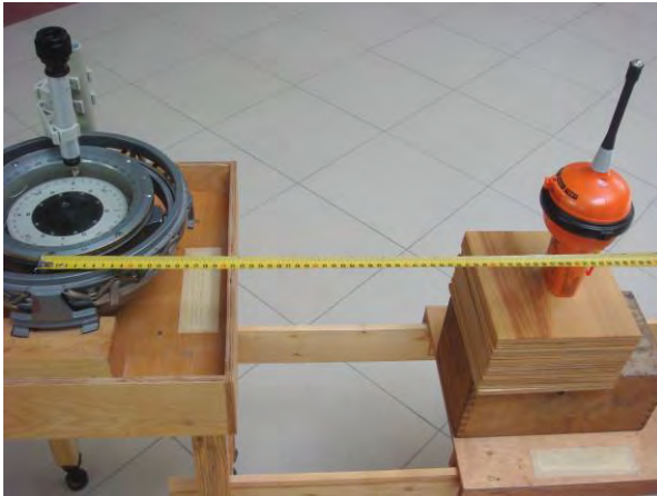
Figure 17.4 – Defining a safe distance from the EPIRB Tron60GPS in vertical position to the main ship's magnetic compass in operational mode. Distance is 0.58 m.
