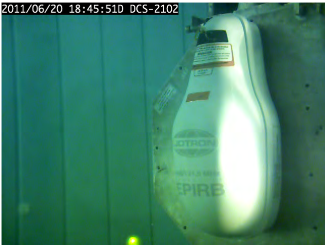
Figure 18.31 – Immersion in the normal mounting position after exposure at temperature +70 °C
