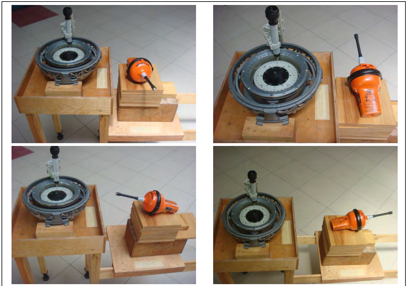
Figure 17.3 – Changing the position EPIRB Tron 60GPS around the horizontal and vertical axis. Maximum deviation search.
