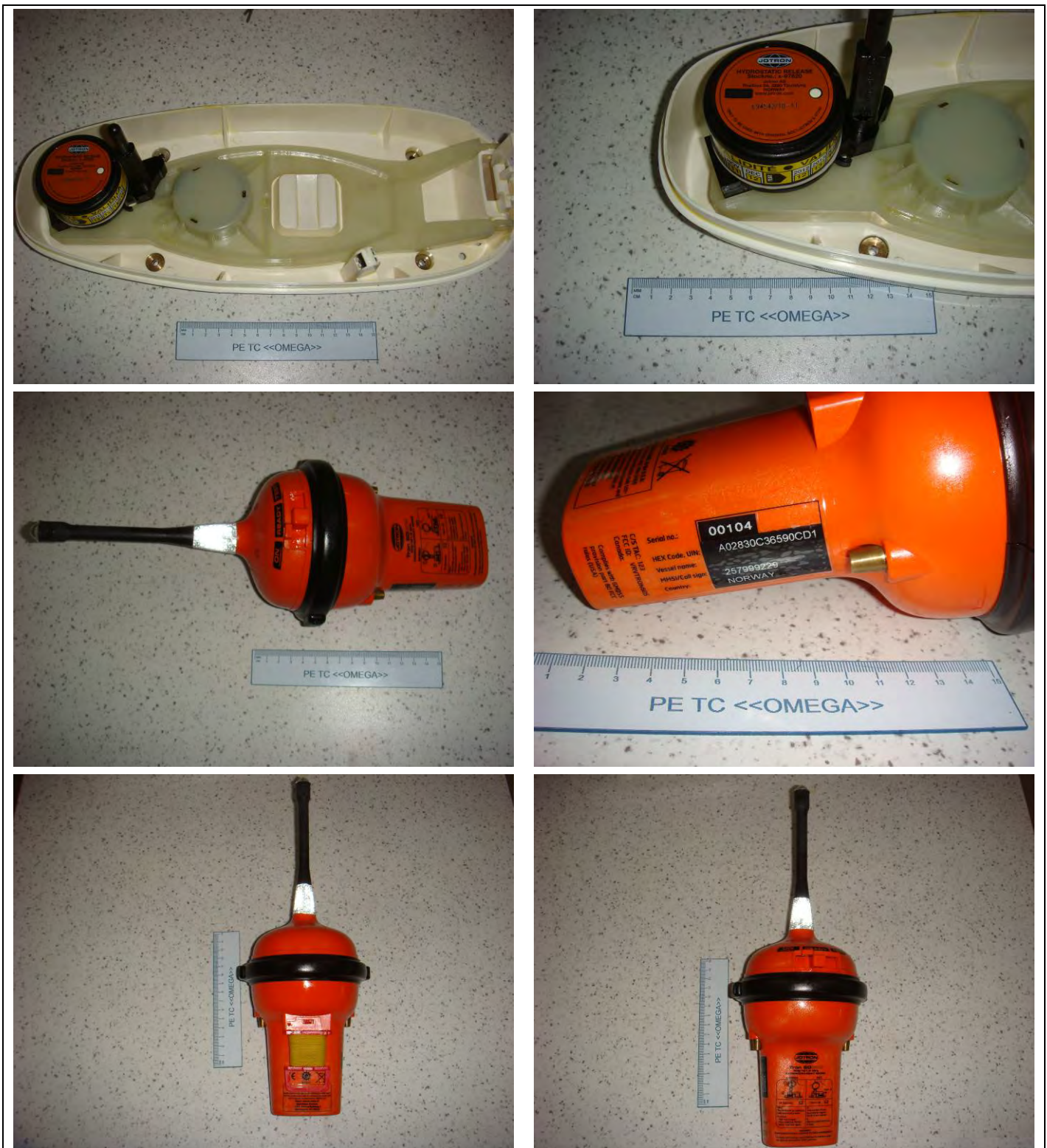
Figure 15.3 - EUT after oil resistance test
