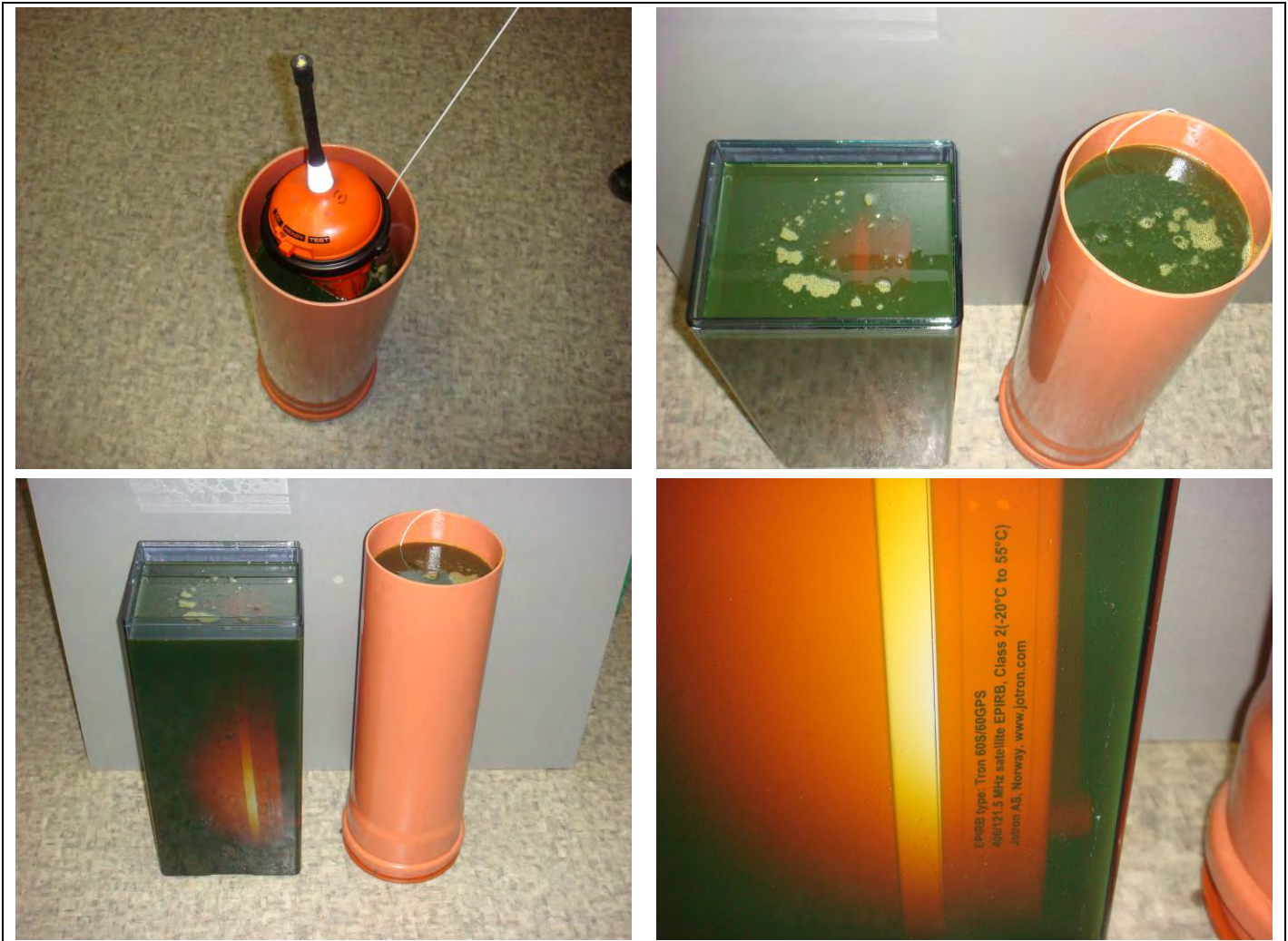
Figure 15.1 - EUT immersing in a tank with oil.
