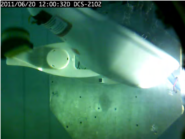
Figure 18.13 – View of automatic release mechanism in Rolling 90° starboard position at the moment of activation
