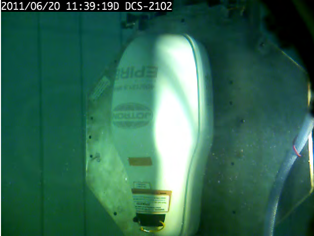
Figure 18.7 – Immersion in the upside-down position
