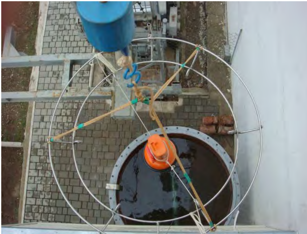
Figure 6.2.4 - EUT dropping in water with antenna vertically down
