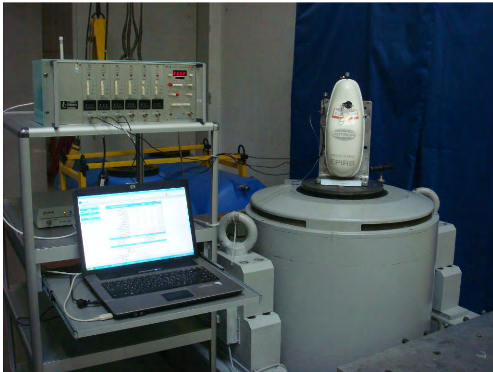
Figure 4.1 - Vibration test in vertical axis Z
