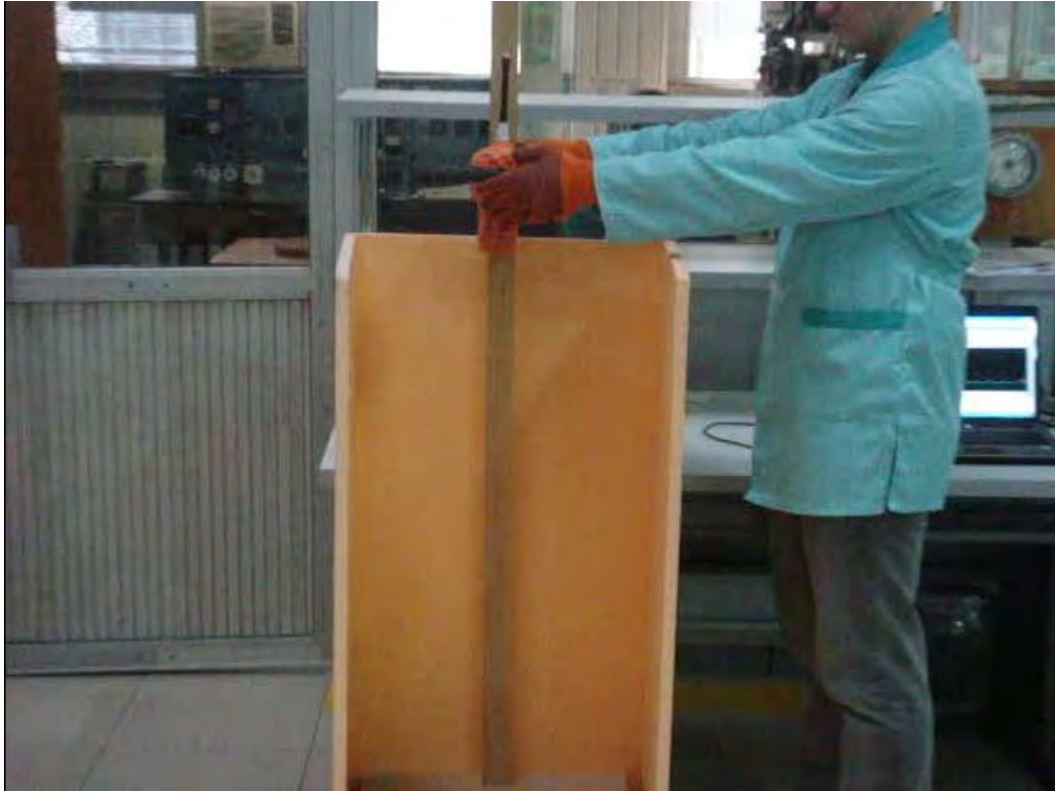
Figure 6.1.1 - Set-up for drop test
