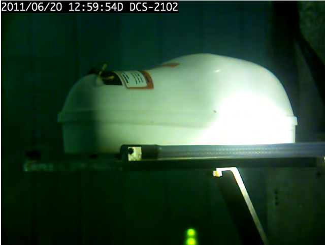
Figure 18.23 – immersion in the pitching 90° stern down position
