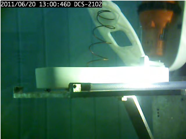
Figure 18.25 – View of automatic release mechanism in Rolling 90° stern down position at the moment of activation
