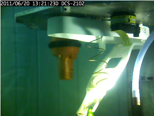
Figure 18.21 – View of automatic release mechanism in Rolling 90° bow down position at the moment of activation
