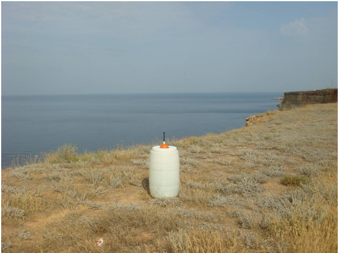
Fig. 5. 3 General view of test site during satellite qualitative test. Conf. 5 - Beacon on water ground plane.
