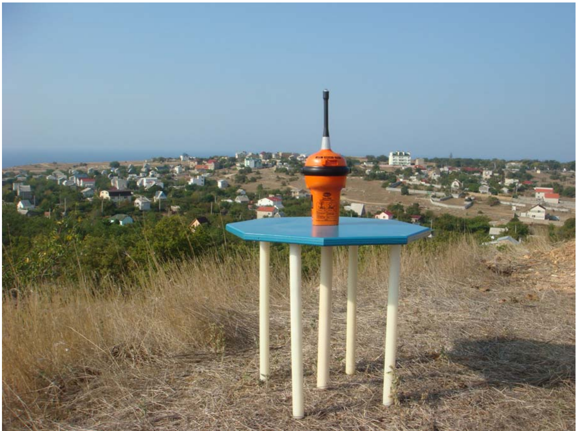
Fig. 5. 4 General view of test site during satellite qualitative test. Conf. 8 – Beacon above ground plane.
