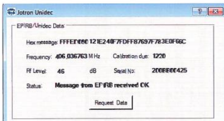
Picture 2. Decoded message shown in the Jotron Unidec PC program.
