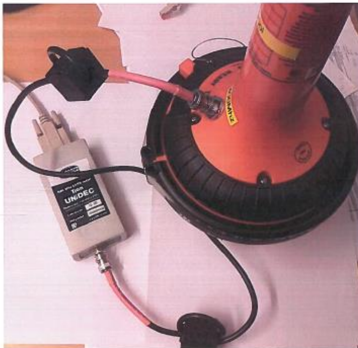
Picture 1. The EUT under test attached to the Unidec tester.
