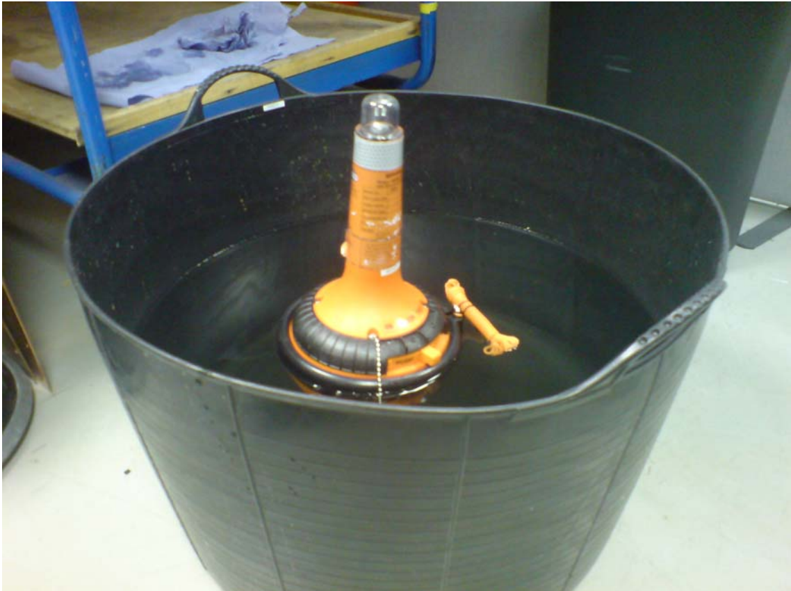
EUT Immersed In Fresh Water
