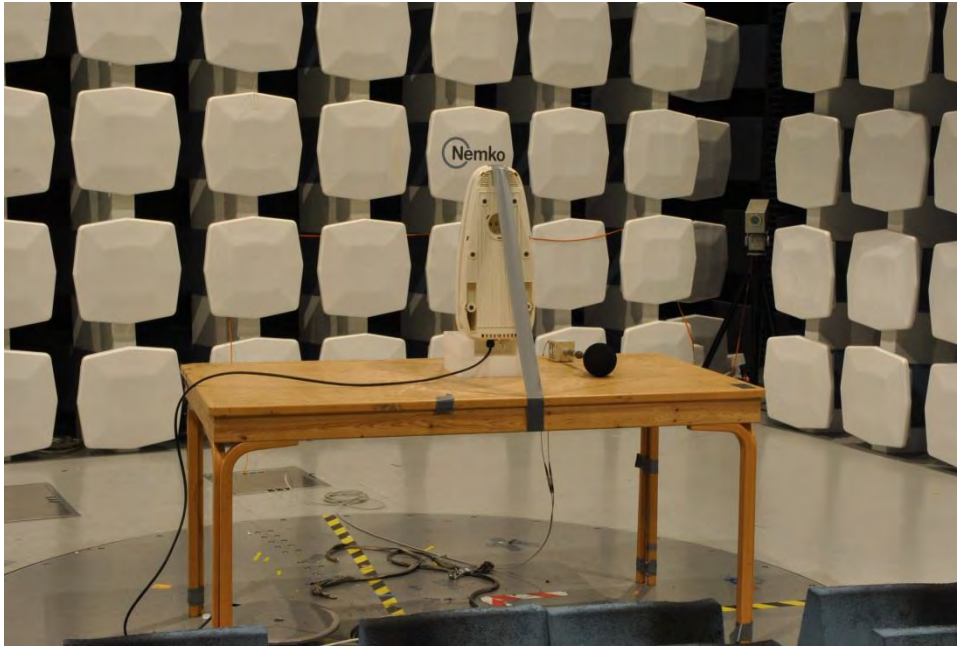
Notes: Test set-up for Radiated RF Field immunity – field immunity was performed without grounding the EUT as this was a worse test
