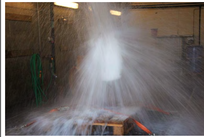
Notes: Test set-up for test to prevent release when water washes over the unit
