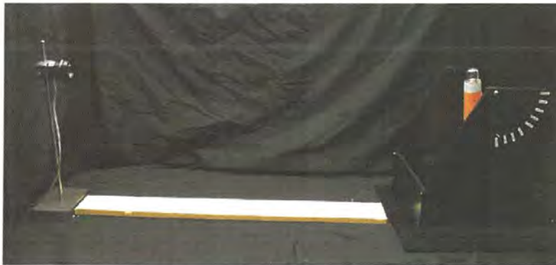
Figure 1.8a Showing test jig and light sensor with lens and a measure stick
