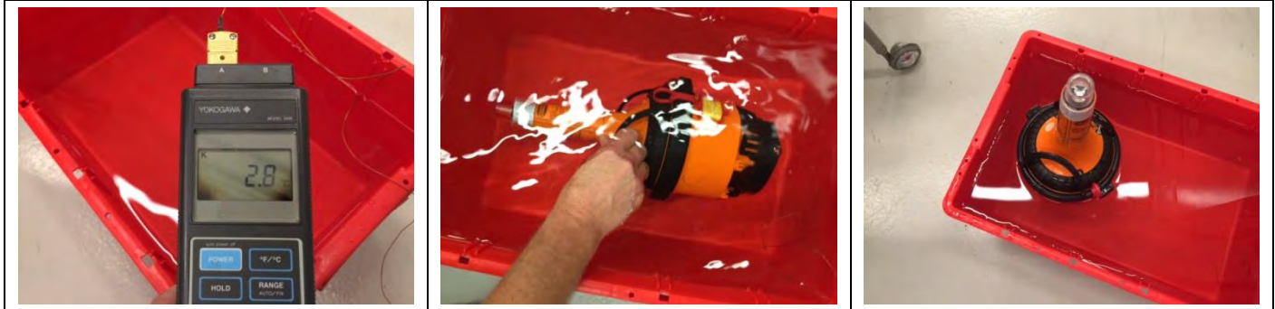
Notes: Test set-up for Thermal Shock Tests
