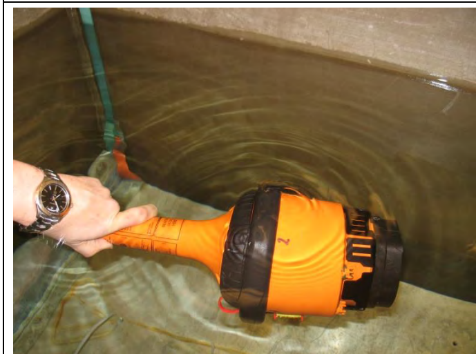
Notes: Test set-up for Stability and Buoyancy tests
