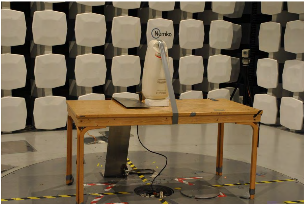
Notes: Test set-up for Radiated Emissions
