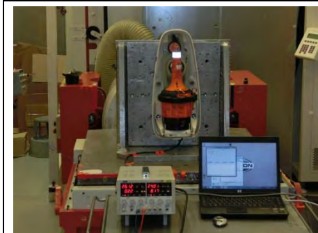
Notes: Test set-up for Vibration and Shock tests ( X, Y and Z)
