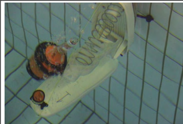
Notes: Test set-up for Automatic release and activation tests
