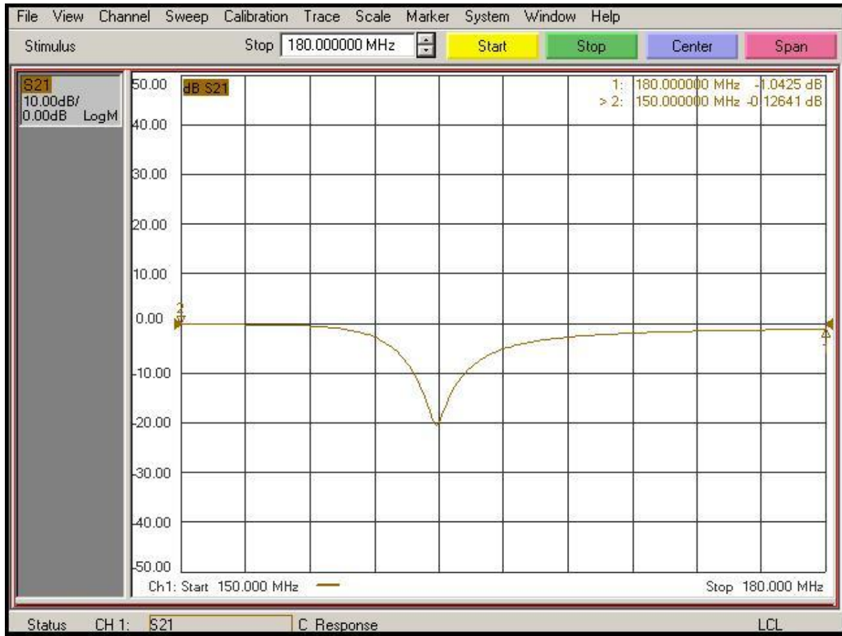
Figure 45: Filter response for the Notch filter applied in some of the measurements of the conducted spurious emissions from the transmitter.
