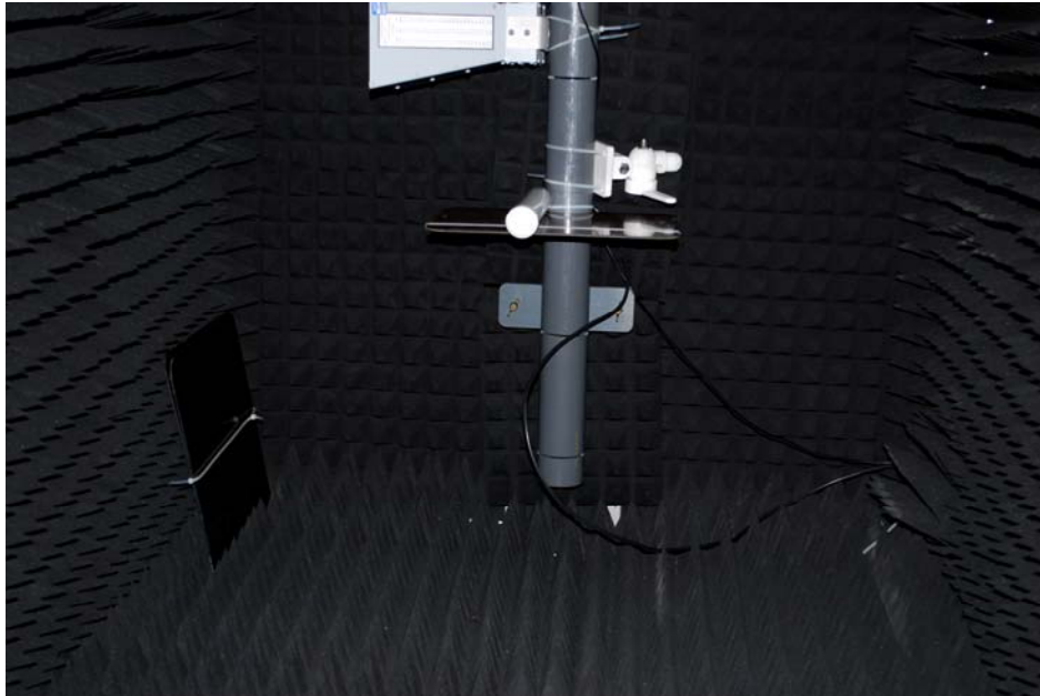
L-Band interference test – GPS antenna unit 2
