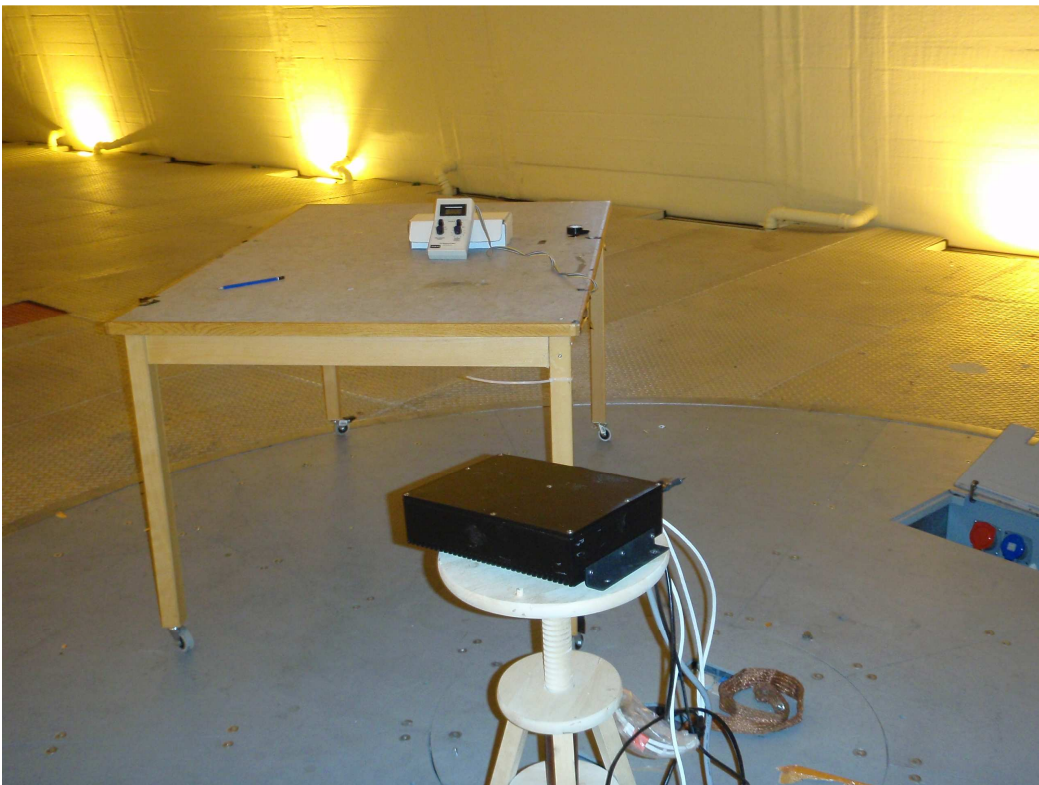
Notes: Test set-up for Compass Safe Distance, Transceiver unit
