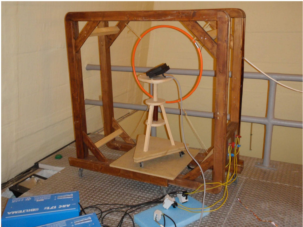
Notes: Test set-up for Compass Safe Distance, Display unit
