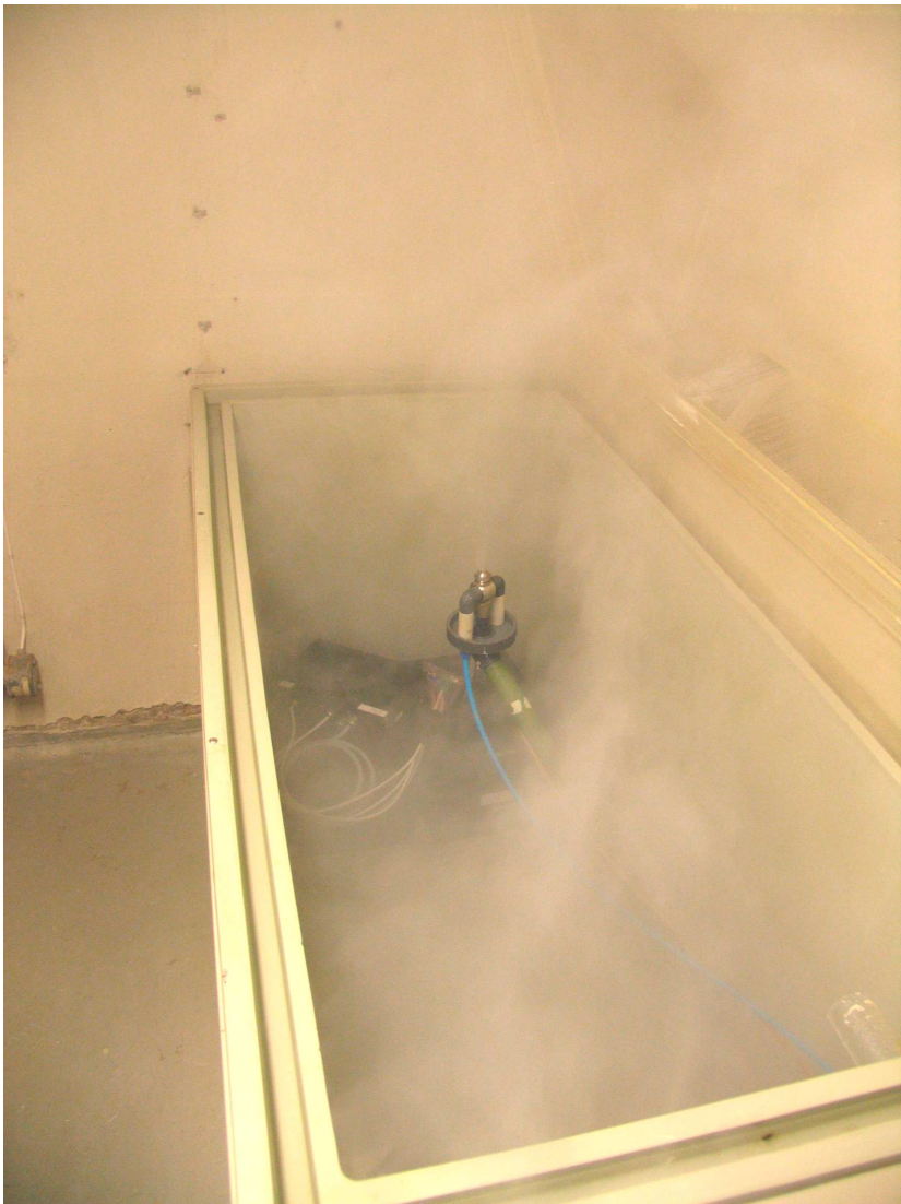
The units in the Salt Mist chamber
